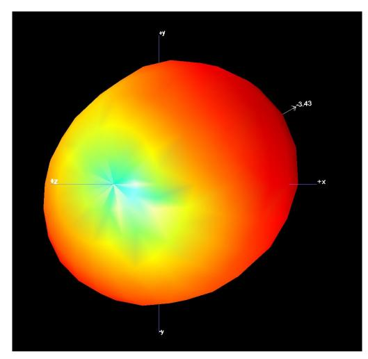
Figure 2a 3-Dimensional Antenna Pattern
