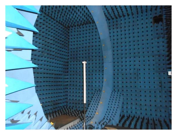
Figure 5a Overall view of SG24L test chamber, showing ring of receiving antennas
