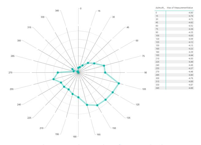
Figure 4 Hearing Aid Antenna Azimuth Cut @ 90 degrees from Z axis. Scale in dBm.
