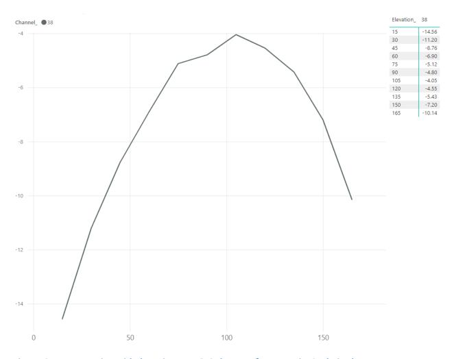
Figure 3 Hearing Aid Elevation cut @ 0 degrees from X axis. Scale in dBm
