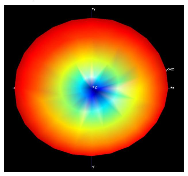
Figure 2 Hearing Aid Antenna Pattern
