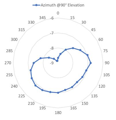
Figure 2b Left Hearing Aid Antenna Azimuth Cut @ 90 degrees from Z axis. Circles are Effective Radiated Power Scale in dBm.
