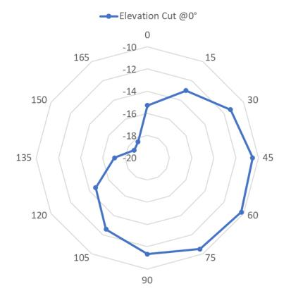
Figure 3b Right Hearing Aid Antenna Azimuth Cut @ 90 degrees from Z axis. Circles are Effective Radiated Power Scale in dBm.
