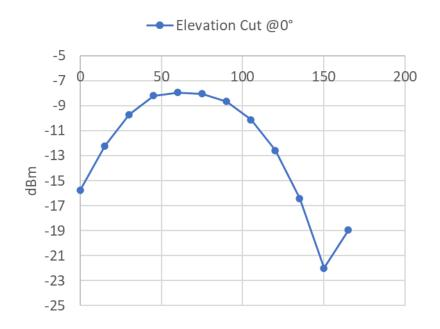
Figure 2a Left Hearing Aid Elevation cut @ 0 degrees from X axis. Y axis Effective Radiated Power Scale in dBm
