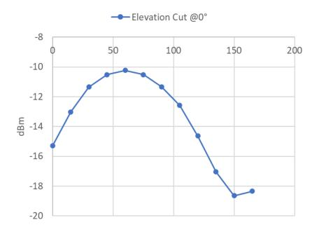
Figure 3a Right Hearing Aid Elevation cut @ 0 degrees from X axis. Y axis Effective Radiated Power Scale in dBm
