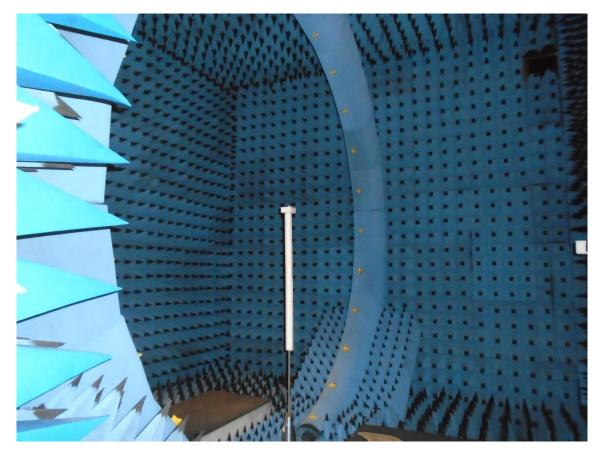
Figure 4a Overall view of SG24L test chamber, showing ring of receiving antennas
