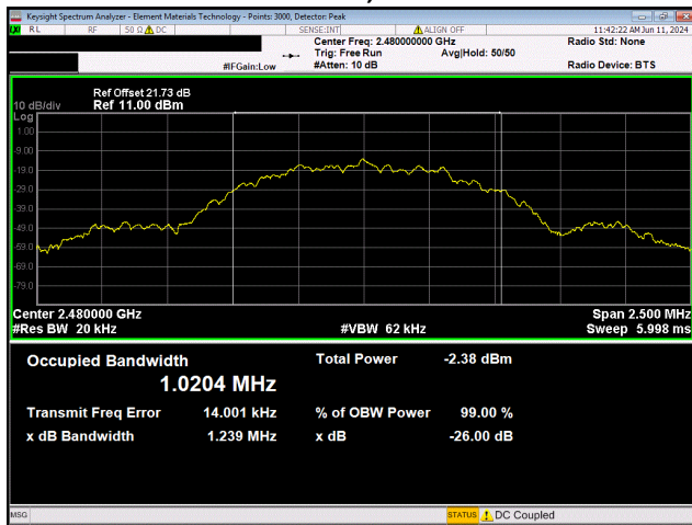
BLE/GFSK 1 Mbps High Channel, 2480 MHz
