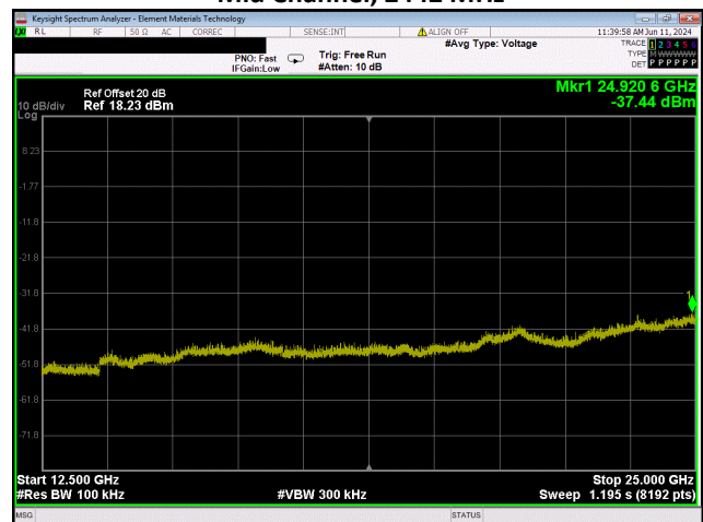
BLE/GFSK 1 Mbps Mid Channel, 2442 MHz
