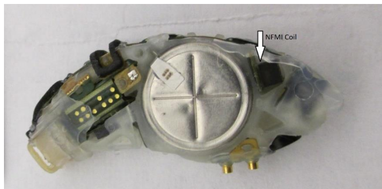
Figure 4c NFMI Antenna in Assembled Hearing Aid
