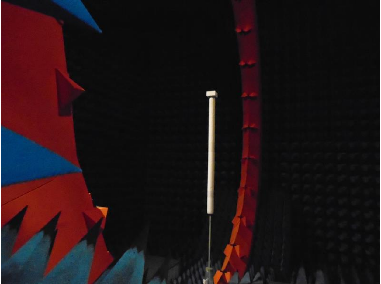
Figure 4a Overall view of SG24L test chamber, showing ring of receiving antennas
