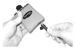
When connected only to the PC via USB, the OBRC will connect with both simultaneous charging and communications - in this case power is pulled from the USB host.
