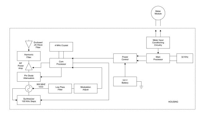
Figure 7 – PET Module Block Diagram
