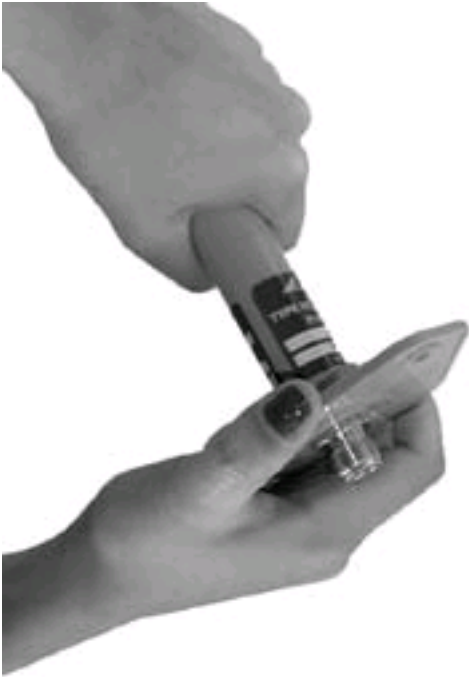
Figure 27 Remote antenna base to remote adapter plate
