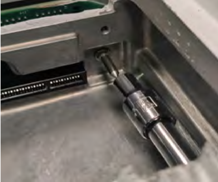
Figure 57 Removing the alignment guide pin
