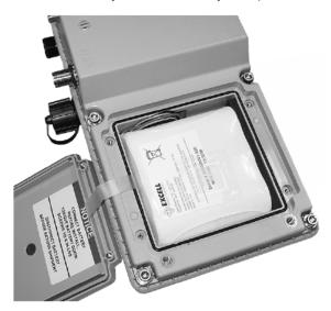
4. Replace the battery compartment cover, and torque the screws to 6 inch-pounds.
