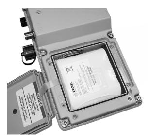
3. Slide the battery into the battery compartment.
