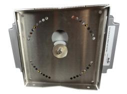
3. Secure the ERT Gateway to the mounting plate using the four set screws.
