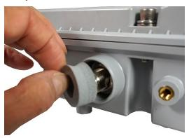
3. Thread the antenna onto the top of the ERT Gateway. Do not over-tighten.
