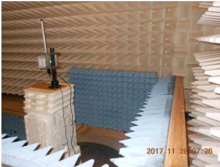
Above 1GHz, 5.15 dBi (150cm), Cone Placement
