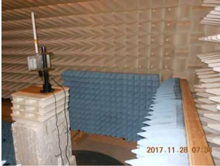
Above 1GHz, 5.5 dBi (150cm), Cone Placement
