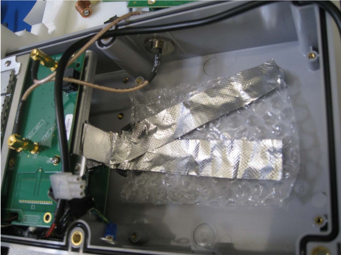
Grounding of the Base Board to the RF Switch Board to reduce radiated emissions.
