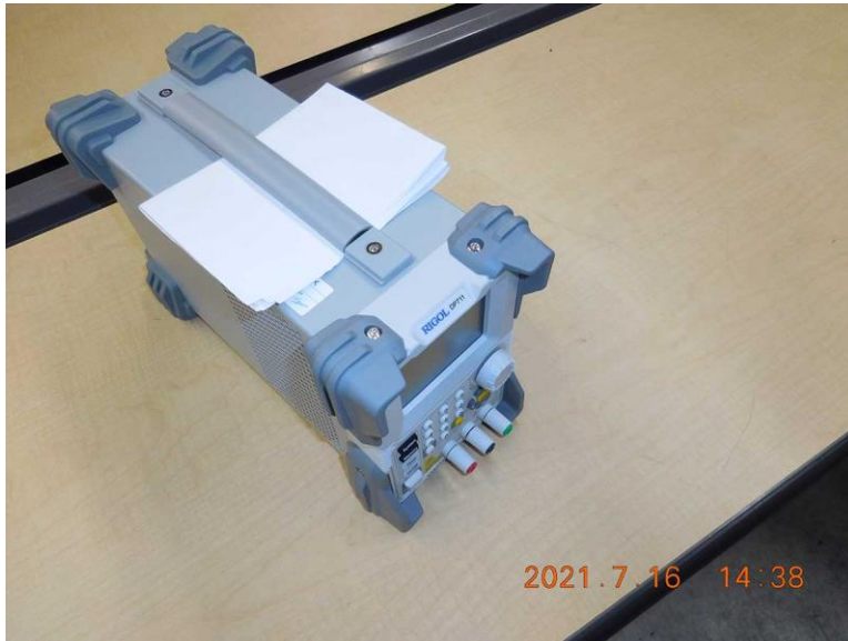
DC Power Supply
