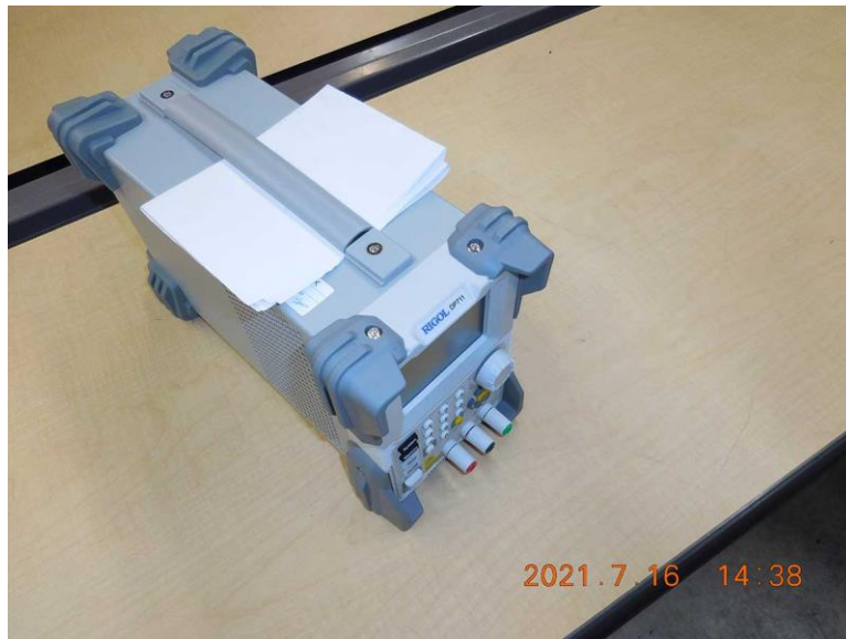
DC Power Supply
