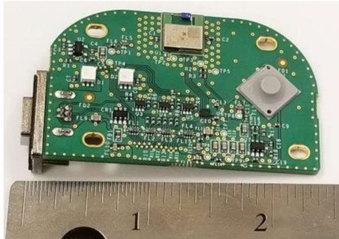
Communications Control Board - Top Side (all devices)
