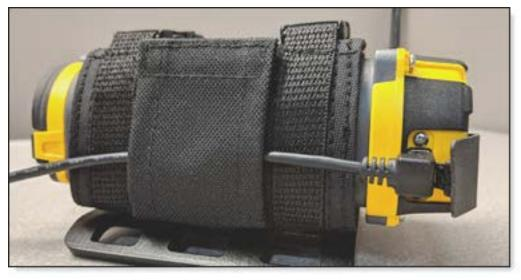
5. Attach the power cable and antenna cable to their connectors on the charge base.
