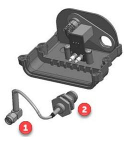
4. Install the new cable and screw the charge base back onto the radio.
