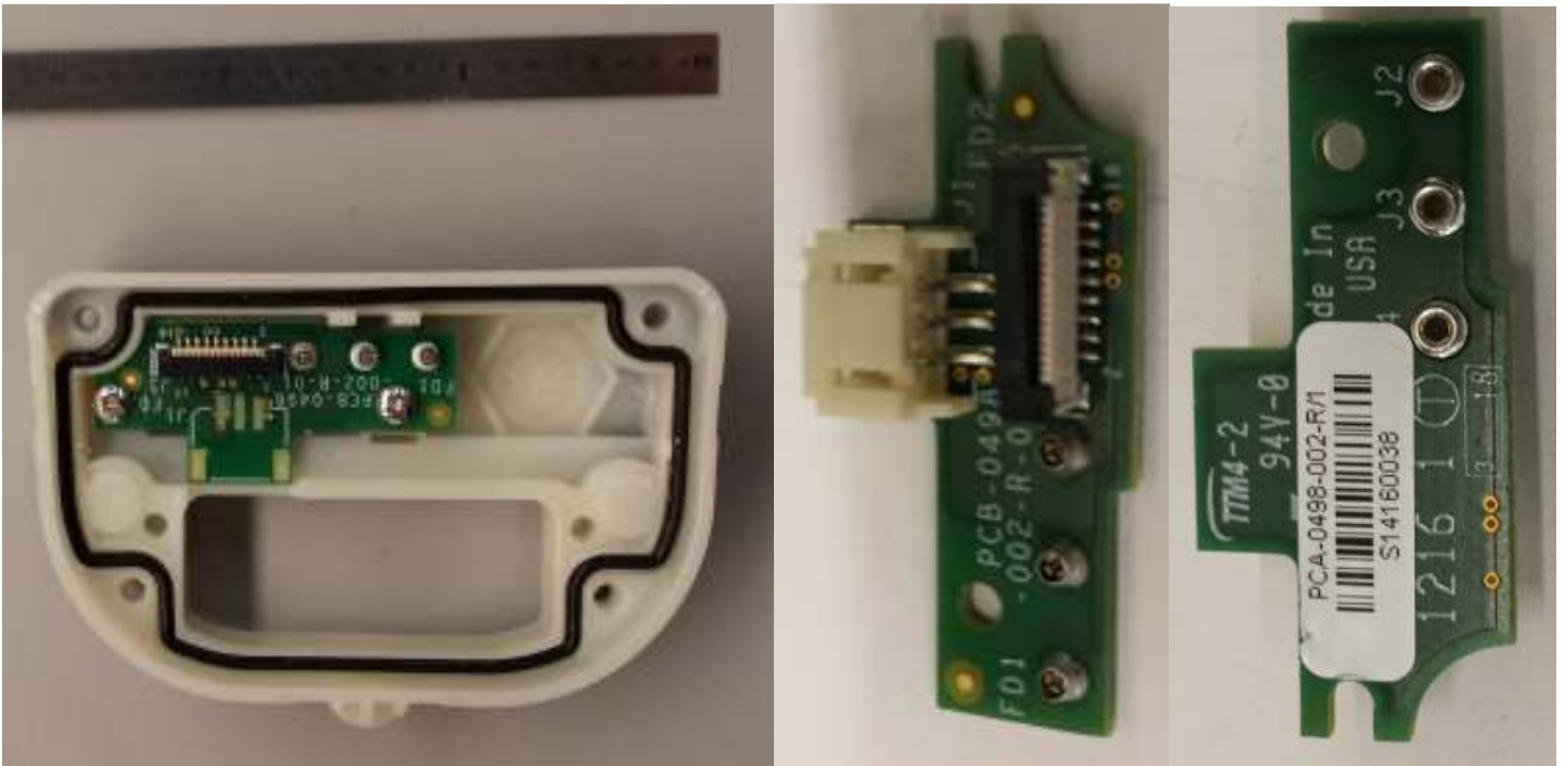
Battery Charger Interface Board PCA-0498-001
