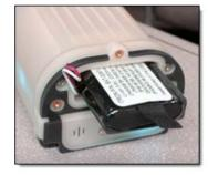
**Caution** Do not pinch the battery wires when replacing the battery compartment cover.
