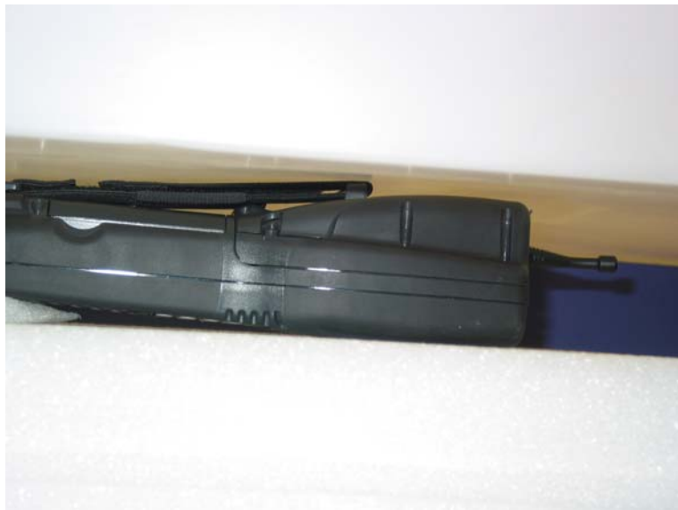
Back Of Unit Test Configuration – Stubby Antenna
