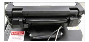
5. When the latch hooks are engaged the latch button on the front of the dock will move into the latched position.
