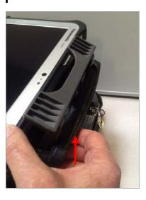
5. When the latch hook is on the top of the tablet, the tablet is now securely latched to the dock.
