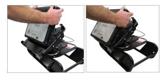
3. Slowly lower the back of the laptop onto the dock, ensuring that the laptop connectors and the dock connectors are aligned. The back of the laptop and the two dock latch hooks should look like this:
