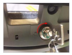
2. Unlock the dock by inserting the dock key into the dock lock and turning it counterclockwise until the lock is in the unlocked position.
