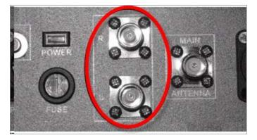
4. Connect the side-looker antenna cables to their respective R (right) and L (left) antenna
