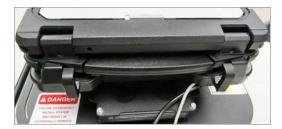
4. Gently push the back of the laptop down onto the dock until the latch hooks snap into place over the rear of the laptop.
