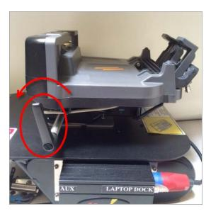
Tilt the tablet dock to the desired position. Rotate the tilt handle towards the top end of the sled to tighten the tablet dock in the desired position.
