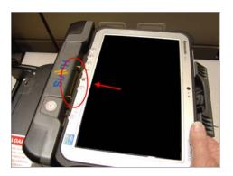
4. Once seated, pull the latch handle up until it snaps in place over the front of the tablet.
