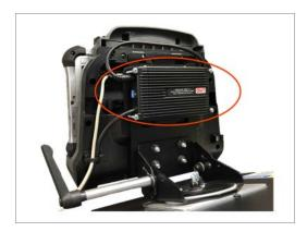
• If needed, plug the red and blue end of the cable into the LAPTOP DOCK receptacle on the junction box.
