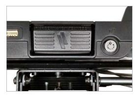
2. Holding the laptop at the top, angle the front edge of the laptop into the dock toward the latch button.
