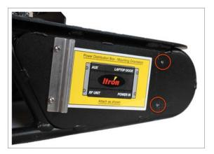
4. Slide one end of the junction box into position over the bracket that is still attached. Be sure to orient the junction box according to the label on the sled or pedestal. The bracket fits into the recessed edge on the junction box.
