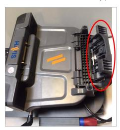
2. Holding the tablet in landscape position, angle the bottom of the tablet towards the dock's connectors.
