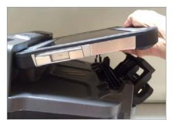
3. Gently push the tablet into the dock's connector and ground pins. Slowly lower the tablet to the dock ensuring that the tablet's connectors and the dock's connectors are aligned.
