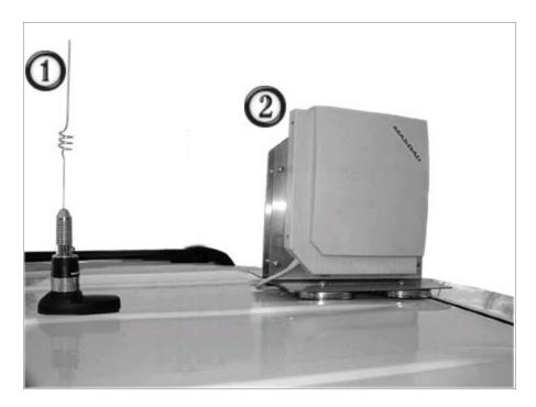
2. Route the antenna cables into the vehicle, taking care not to pinch or damage them.
