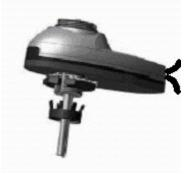
Antenna Element: Center Frequency: 1575.42 MHz ±1.023 MHz Output Impedance: 50 Ohm Current consumption: 12 mA max Amplified Gain: 26dB min Radiation Pattern Omni Dimensions: 2.25" W x 4.25" L x 1.25" H Cable: RG174 (GPS antenna side) 17' RG58/U (mobile antenna side) Connectors: GPS Connector: Male SMA (MSMA) Male TNC Mobile Connector:
