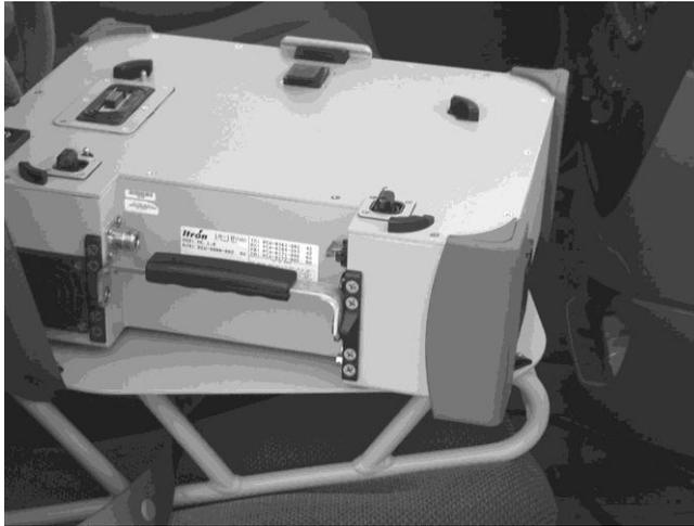
3. While gently applying downward pressure, rotate the collector back and forth slightly until the three pins on the base fit into the three matching holes on the underside of the Mobile Collector.
