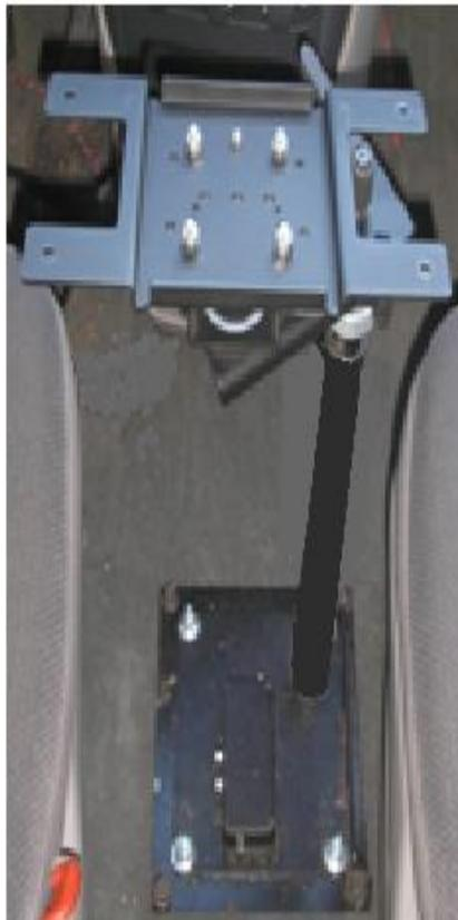
2. Place the mount and brackets for the power distribution box in the middle of the pedestal. Tighten securely.
