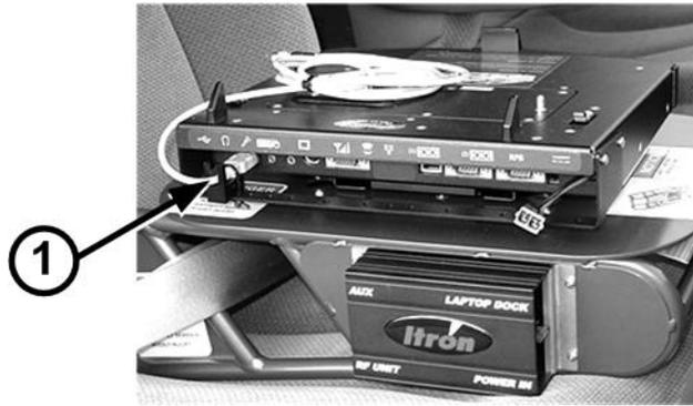
2. Plug the round end of the USB cable into the MC3 radio by pulling the connector sleeve back, plugging the connector in to the receptacle, and releasing the sleeve.
