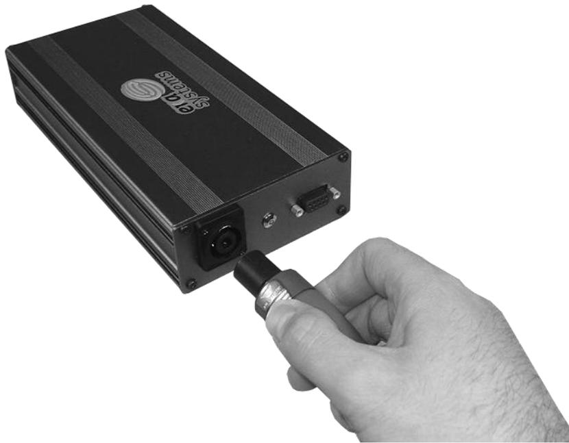
9. Connect the serial cable to COM 1 serial port on the laptop (or dock); this is the end without pins. Be sure to securely connect the cable.
