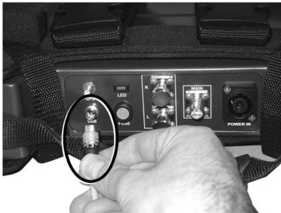
5. Connect the antennas and power cables for the MC3 as described earlier in this document.
