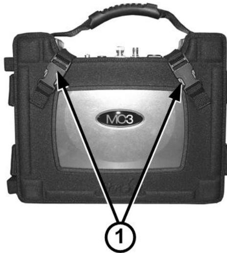
2. Strap the mount to either the front or the back of the passenger-side seat back. Position the unit within the mount so that when it is strapped to the seat back, the unit's connectors face *toward the passenger-side door*.
