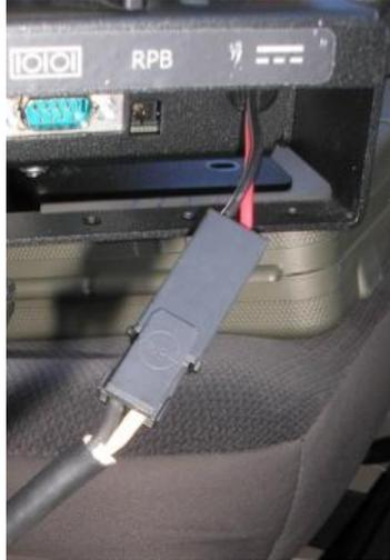
2. Connect the other end of the CBA-0187-004 cable. This cable will come pre-wired to the vehicle dock with a clip to hold the cable in place.
