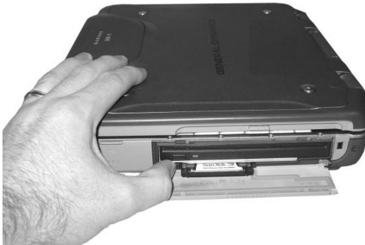
3. Pull the adapter the rest of the way out.
