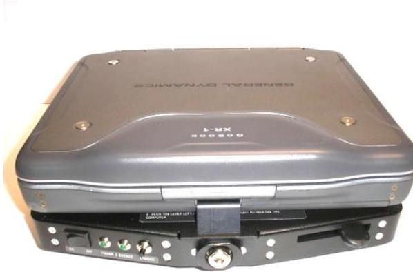
3. Push the locking lever in and to the right to secure the laptop on the dock.
