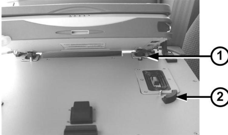
4. Insert the key into the mounting lock and press the locking mechanism so it engages the GoBook MAX.
