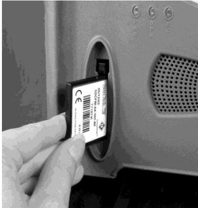
2. Insert the card in the flash card reader slot and press it in until it is firmly in place and the eject button pops out.
