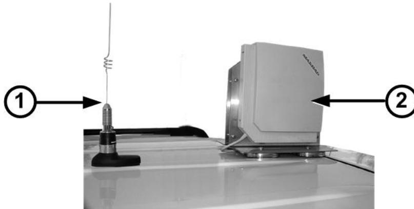
2. Route the antenna cables into the vehicle.
