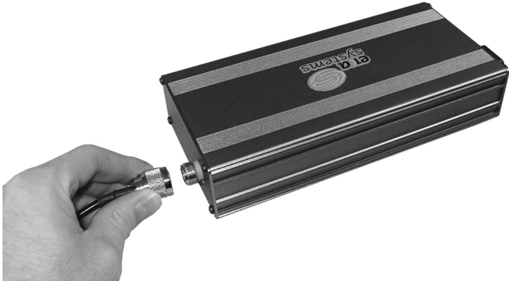
7. Connect the EkaNet power cable to the **AUX** port on the junction box in your vehicle.
