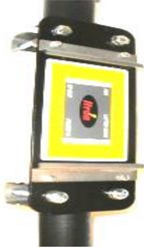
3. Remove the two screws in the top mounting bracket.
