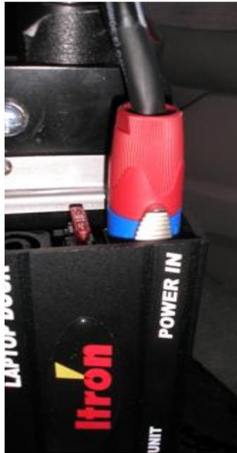
2. Use the CBA-0269-001 cable to connect the power distribution box to the RF unit in the **RF Unit** slot.
