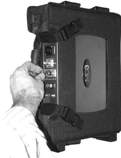
4. Connect the side-looker antenna cables to the R and L antenna inputs on the MC3 radio.
