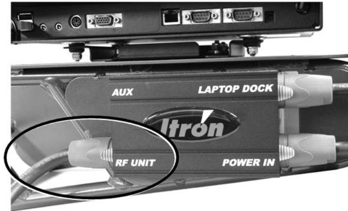
2. Plug the other end into the **POWER IN** receptacle on the MC3.
