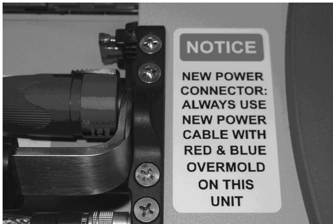
The operation of the new power cable is slightly different from the previous power connector. To engage the new power connector, align the connector tab with the connector slot on the RF unit, insert the connector and then rotate clockwise 45 degrees. To disengage the unit, pull back the locking tab on the cable connector and then rotate the connector 45 degrees counterclockwise. Notice labels were placed on both ends of your power cable to remind you how to disengage the new power connector.
