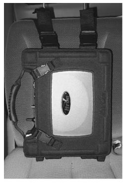
3. Tighten the straps until the RF unit is snug against the seat back.
