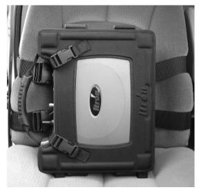
• Bench seat – connect the optional bench-seat straps to the buckles on the bottom of the vehicle mount.
