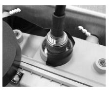
c. Wrap the vinyl electric tape up the coaxial cable overlapping each wrap as shown in the following illustrations.
