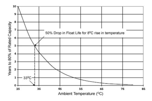
A ten year battery lasts for five years at  $33^{\circ}$ C (91.4°F) and only  $2\frac{1}{2}$  years at  $41^{\circ}$ C (105.8°F).
