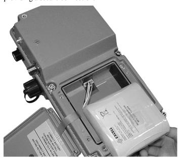
3. Slide the battery into the battery compartment.
