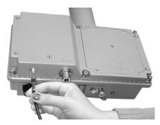
The WAN cable has an N connector on each end. Connect one end of the WAN antenna cable to the CCU. Connect the other end of the cable to the external WAN antenna.
