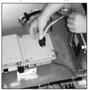
6. Feed the GPS and WAN (if required) antenna cables through the Roxtec block and connect them to the CCU.
