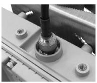
b. Wrap vinyl electrical tape around the connection starting at the CCU and wrapping up the cable as shown in the following illustration.
