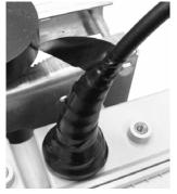
g. Continue wrapping the vinyl tape in a spiral back down to the CCU. You now have two layers of vinyl tape covering the butyl rubber.
