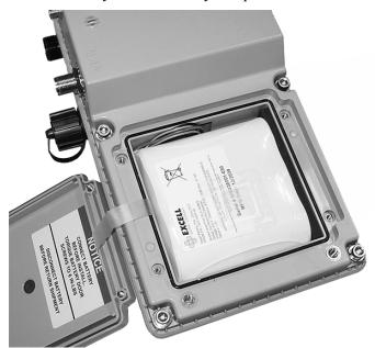
4. Replace the battery compartment cover, and torque the screws to 6 inch-pounds.
