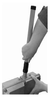
3. Push the rubber boot as close as possible to the top of the CCU as shown in the following illustration.
