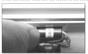
4. Place the battery in the battery well as shown in the following illustration.
