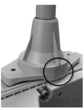
5. Using the included screws and washers, screw the antenna sleeve to the top of the CCU/Repeater. Tighten the screws to 5 to 6 in/lbs.
