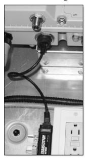
Connect the battery to the connector on the battery door of the CCU.
