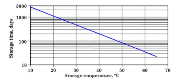
When batteries are stored at or near 25°C (77°F) it is recommend to conduct an open circuit voltage (OCV) audit every six months and recharge when OCV readings approach 6 volts (2.00 volts per cell). If storage temperatures are significantly higher than 25°C (77°F), even for short durations, the frequency of OCV audits must increase.
