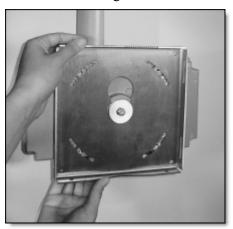
4. Using the provided set screws, secure the CCU to the mounting plate with the antenna in the upright position.
