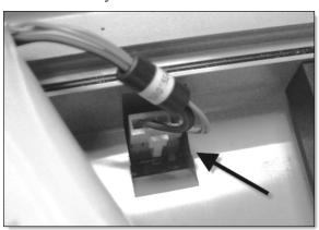
2. Align the edges of the ferrite bead with the edges of the recess in the battery well.
