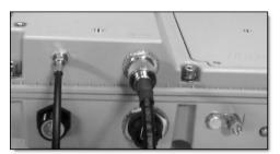
7. Connect the power cable to the CCU.
