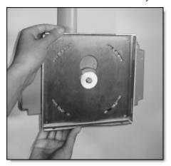
4. Using the provided set screws, secure the CCU to the mounting plate with the antenna in the upright position.
