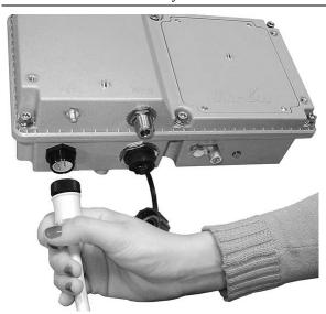
2. Securely fasten the power cable to the CCU/Repeater by tightening the retaining nut on the cable.
