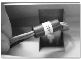
3. Press the ferrite bead into the recess in the battery well.
