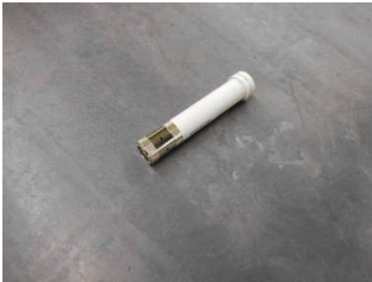
Attached WAN Antenna
