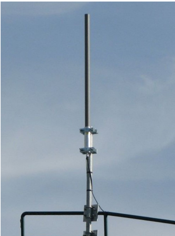
Remote 8.15 dBi 915 MHz antenna: 68.0" L x 2.0" D
