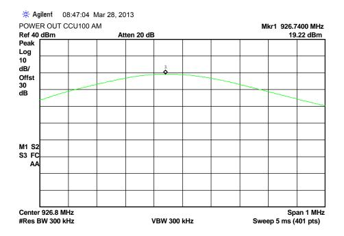
Note 1: This variance is due to the path loss from the internal CCU100 cavity filter. Path loss of this filter is specified as 5.0 dB max from 924MHz to 926MHz and 12dB min at 928 MHz.
