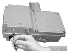
2. The WAN cable has a TNC connector on one end and an N connector on the other end. Connect the N connector end of the WAN antenna cable to the CCU. Connect the TNC end of the cable to the remote WAN antenna.
