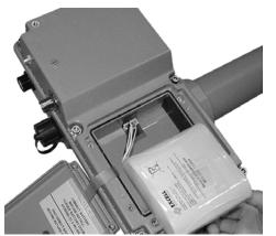
3. Slide the battery into the battery compartment.
