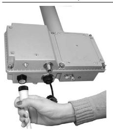
2. Securely fasten the power cable to the CCU/Repeater by tightening the retaining nut on the cable.
