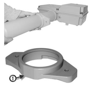
3. Using the included screws, washers, and lock washers, screw the antenna sleeve to the top of the CCU/Repeater. Tighten the screws to 5 to 6 in/lbs.
