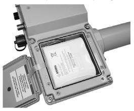
4. Replace the battery compartment cover, and torque the screws to 6 inch-pounds.
