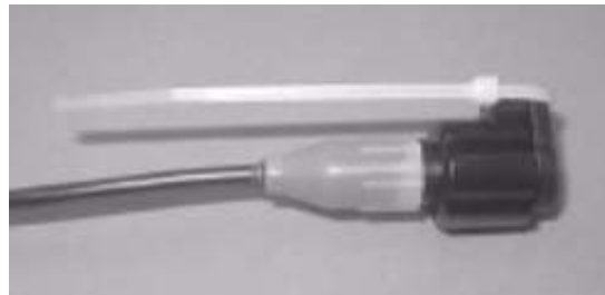
Figure 10: Cable tie on register connector
