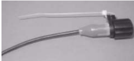
Figure 10: Cable tie on register connector
