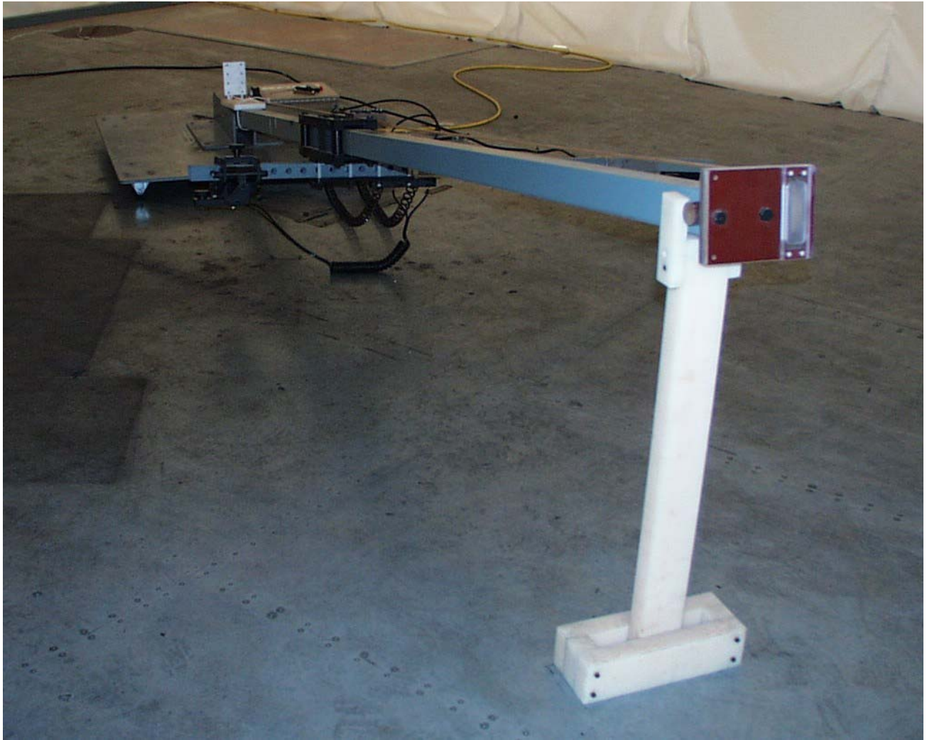
Photo 19 Antenna Mast in Holder / Cradle
