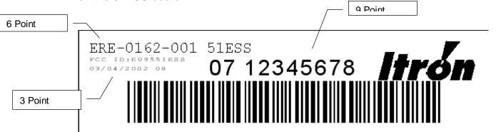
The following label will be placed on the 51ESS board:
