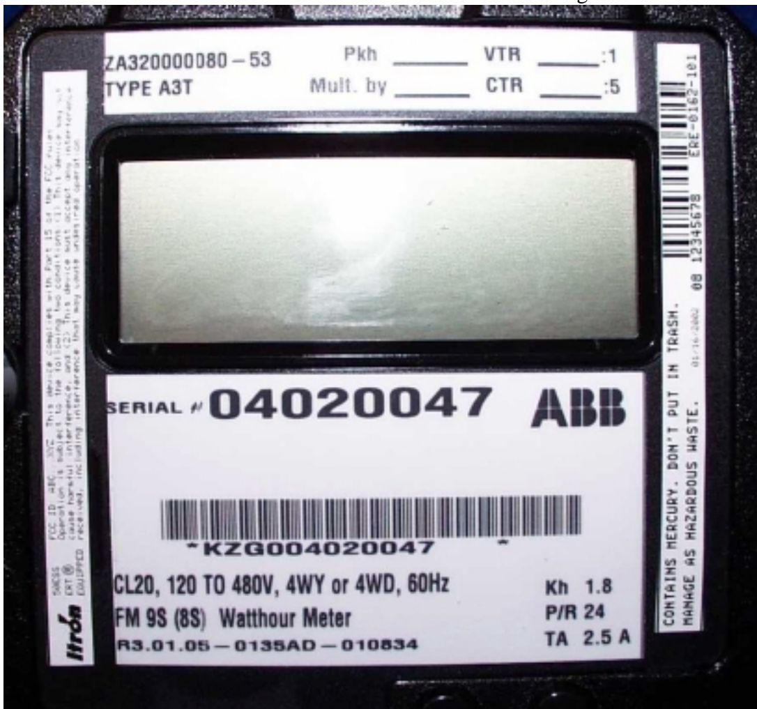
Labels attached to the Internal Meter Housing
