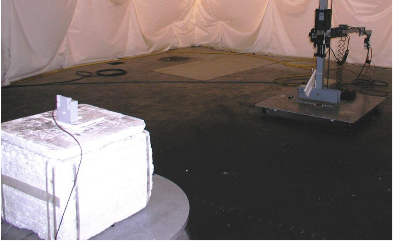
Figure 21: Test setup for radiated spurious emissions above 18GHz (vertical polarity) shown with Remote in upside down position.
