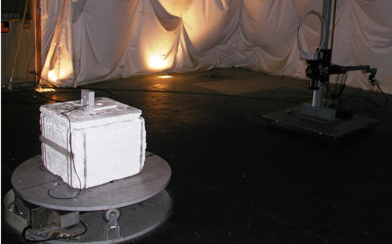
Figure 3: Test setup for radiated spurious between 9kHz and 30MHz with Loop Antenna shown and Remote in upright position.
