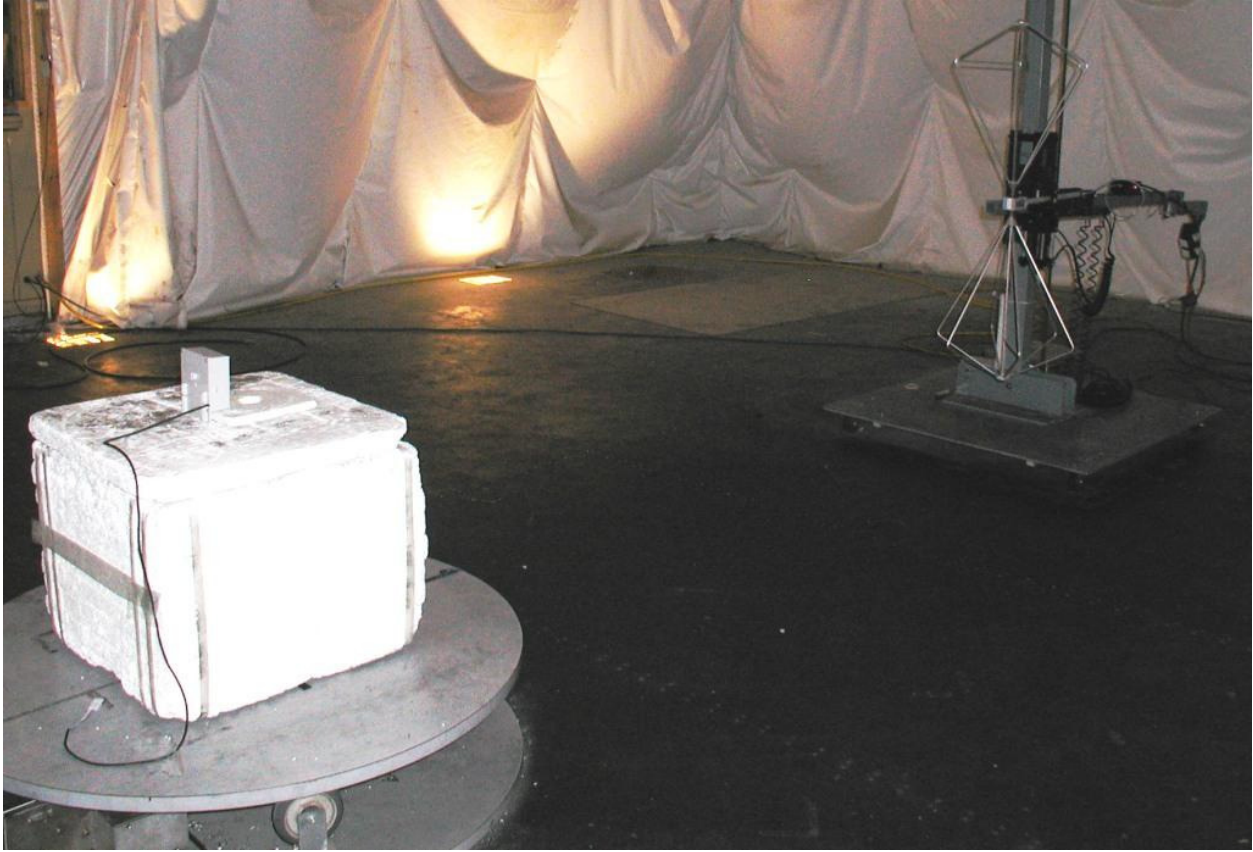
Figure 7: Test Setup for Radiated Spurious measurements between 30MHz and 300MHz using Biconical antenna shown here in vertical orientation and Remote in upright position.
