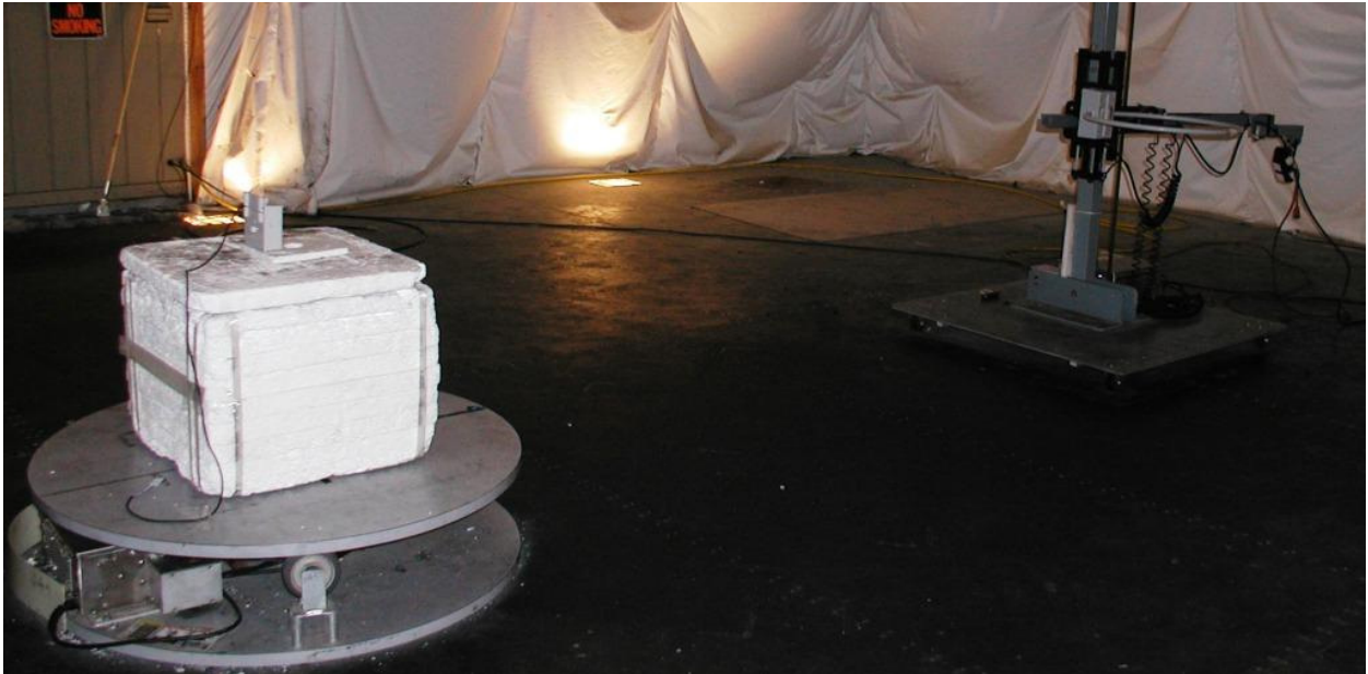
Figure 4: Test setup for radiated spurious between 9kHz and 30MHz with Loop Antenna and Remote in upside down position.
