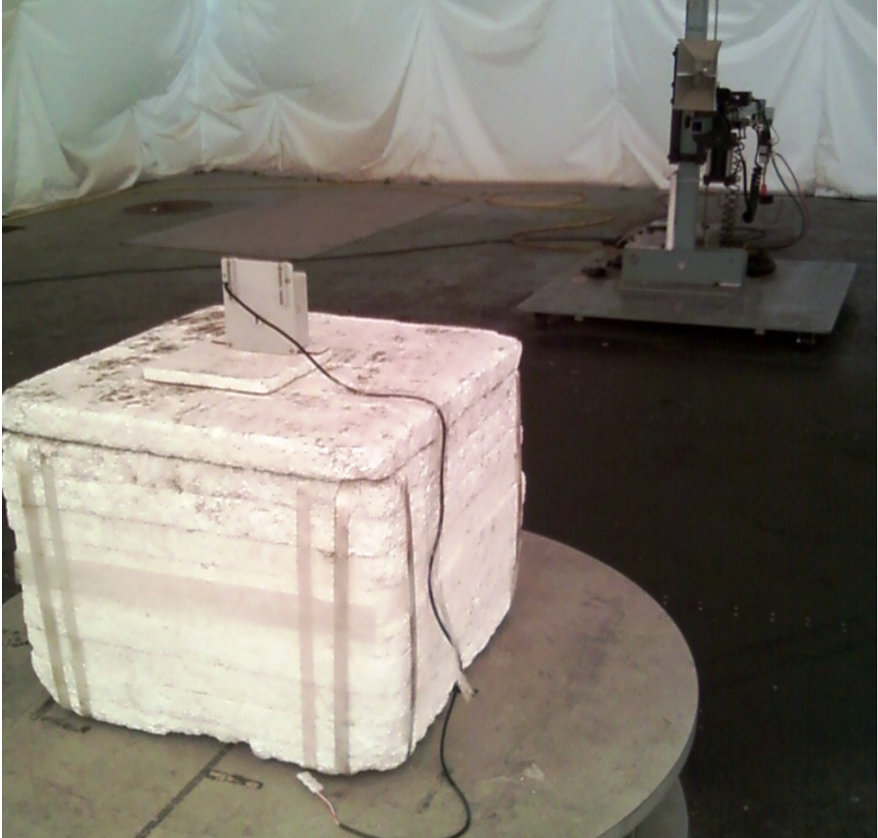
Figure 13: Test setup for radiated spurious emissions below 18GHz with horn in horizontal polarity and Remote in upside down position.
