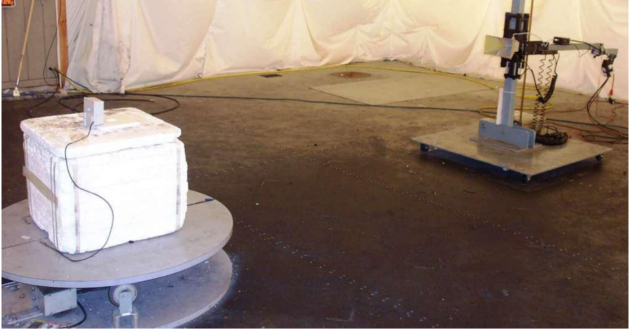
Figure 14: Test setup for radiated spurious emissions below 18GHz with horn antenna in vertical polarity and Remote in upright position.
