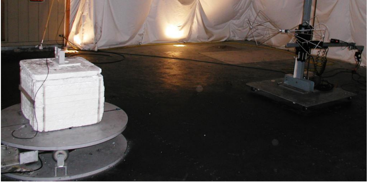
Figure 6: Test Setup for Radiated Spurious measurements between 30MHz and 300MHz using Biconical antenna shown here in horizontal orientation and Remote in upside down position.
