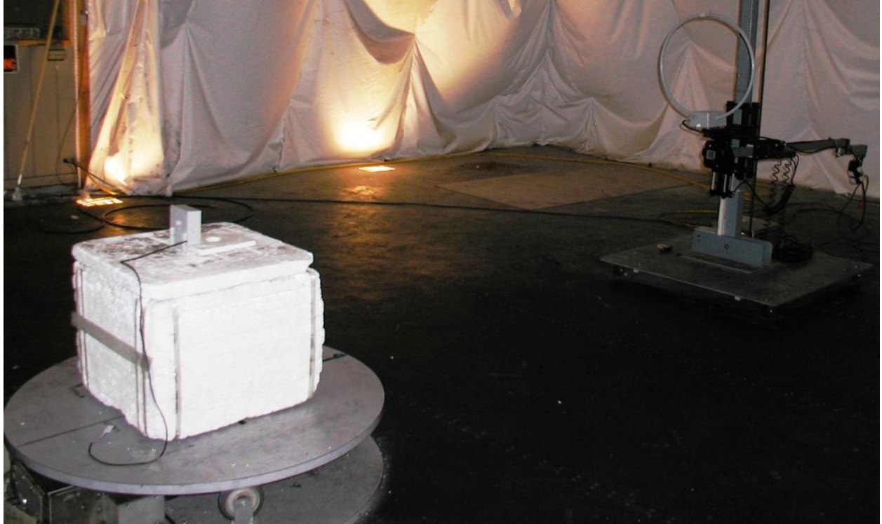
Figure 2: Test setup for radiated spurious between 9kHz and 30MHz with Loop Antenna shown and Remote in upright position.
