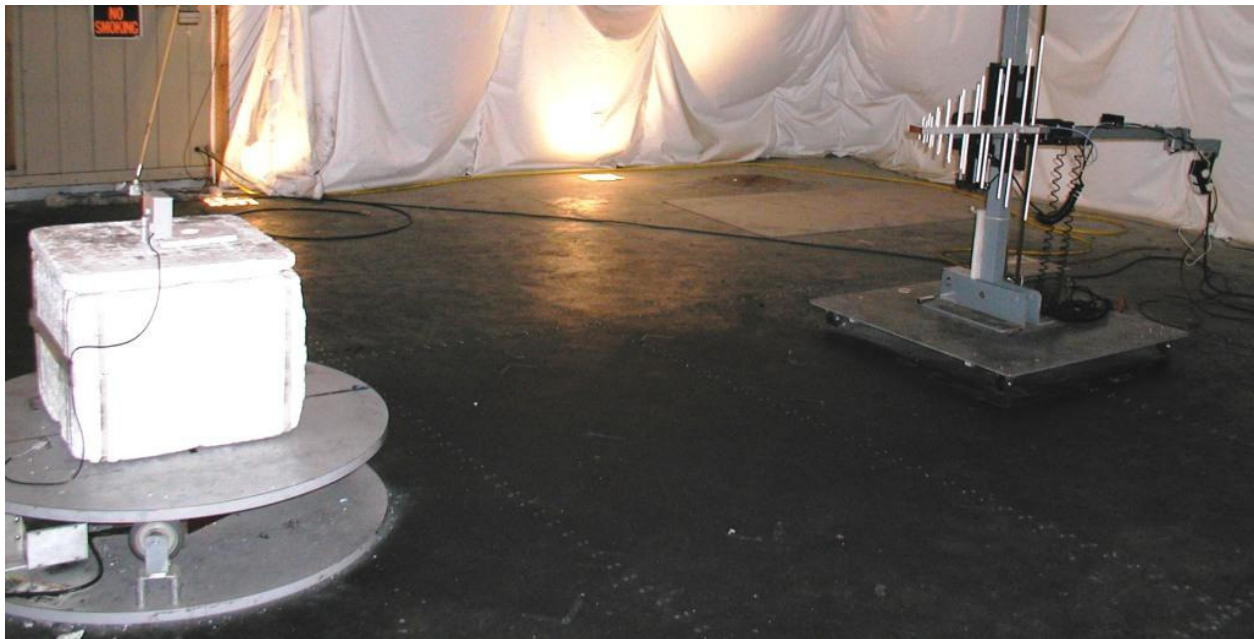
Figure 10: Test setup for TX radiated spurious between 200MHz and 2GHz with Log Periodic in vertical orientation shown with remote in upright position.
