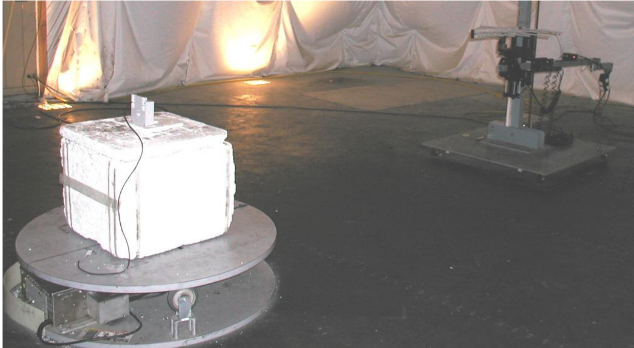
Figure 9: Test setup for RX radiated spurious between 200MHz and 2GHz with Log Periodic in horizontal orientation shown with Remote in upside down position.
