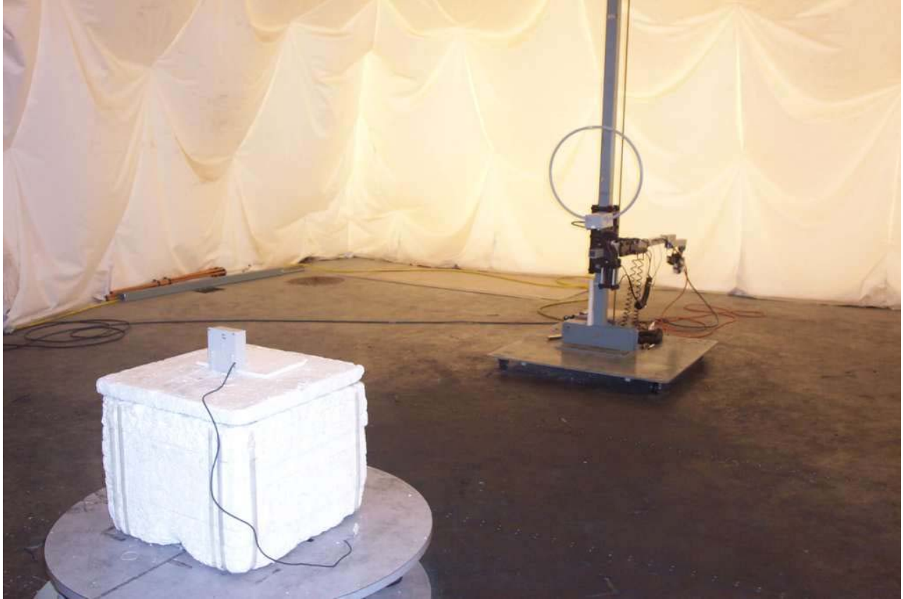
Figure 2: Test setup for radiated spurious between 9kHz and 30MHz with Loop Antenna shown with Remote.
