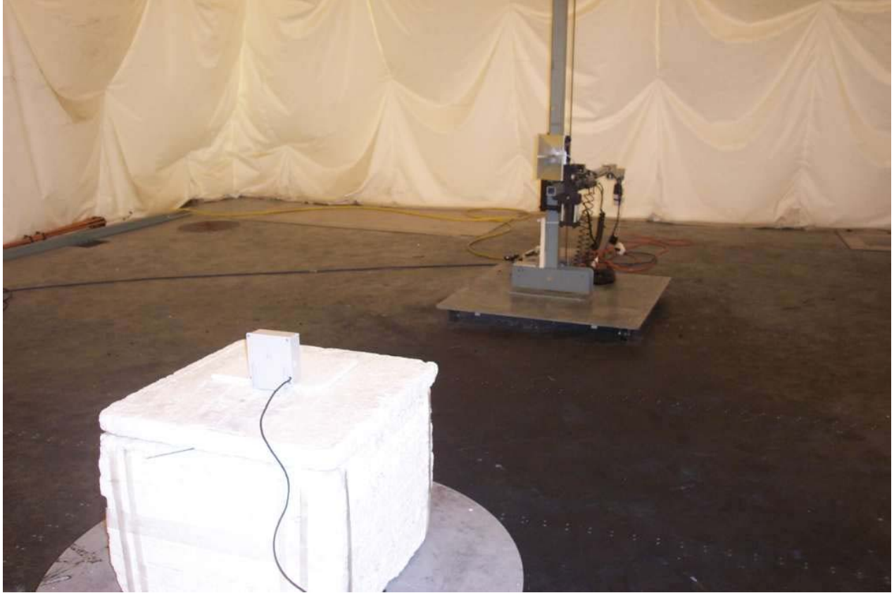
Figure 13: Test setup for radiated spurious emissions below 18GHz with horn in horizontal polarity and Remote on turntable
