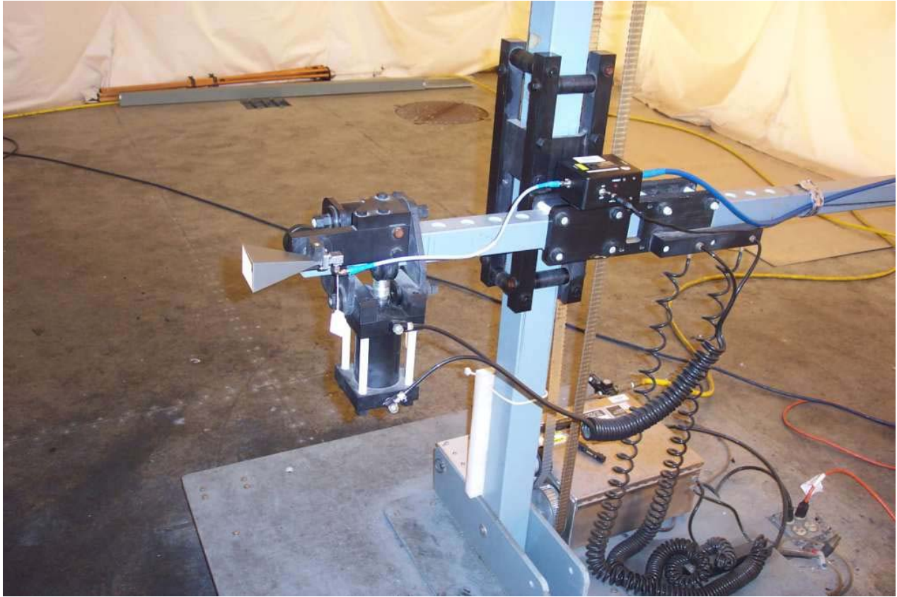
Figure 21: Test setup for radiated spurious emissions above 18GHz (Vertical polarity shown)
