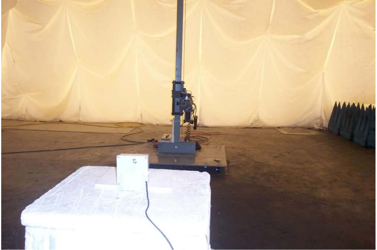
Figure 20: Test setup for radiated spurious emissions above 18GHz (Horizontal polarity) shown with Remote on turntable
