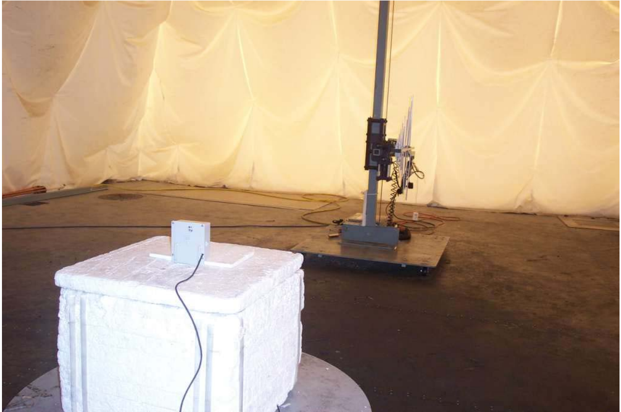
Figure 9: Test setup for radiated spurious between 200MHz and 2GHz with Log Periodic in vertical orientation shown with remote in foreground
