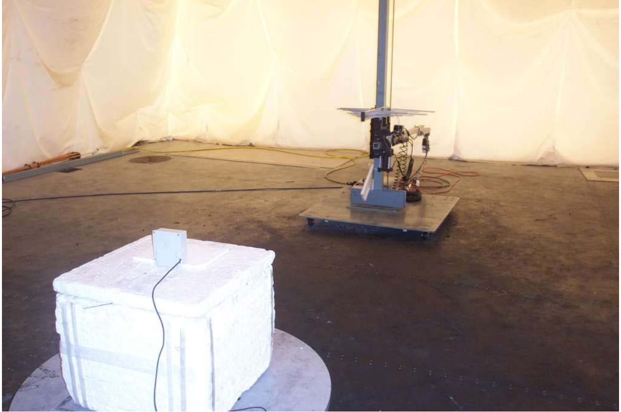
Figure 8: Test setup for radiated spurious between 200MHz and 2GHz with Log Periodic in horizontal orientation shown with remote in foreground
