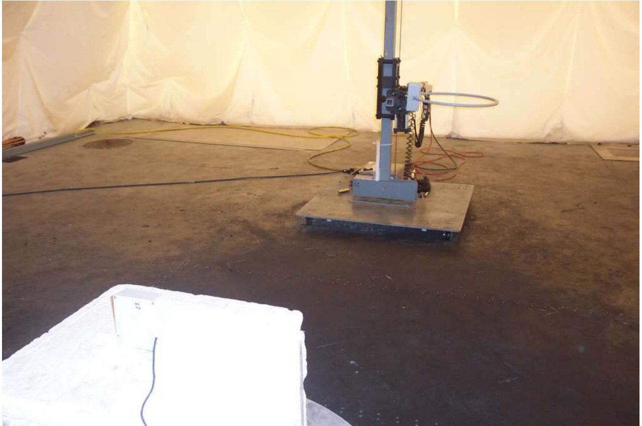
Figure 4: Test setup for radiated spurious between 9kHz and 30MHz with Loop Antenna shown with Remote.
