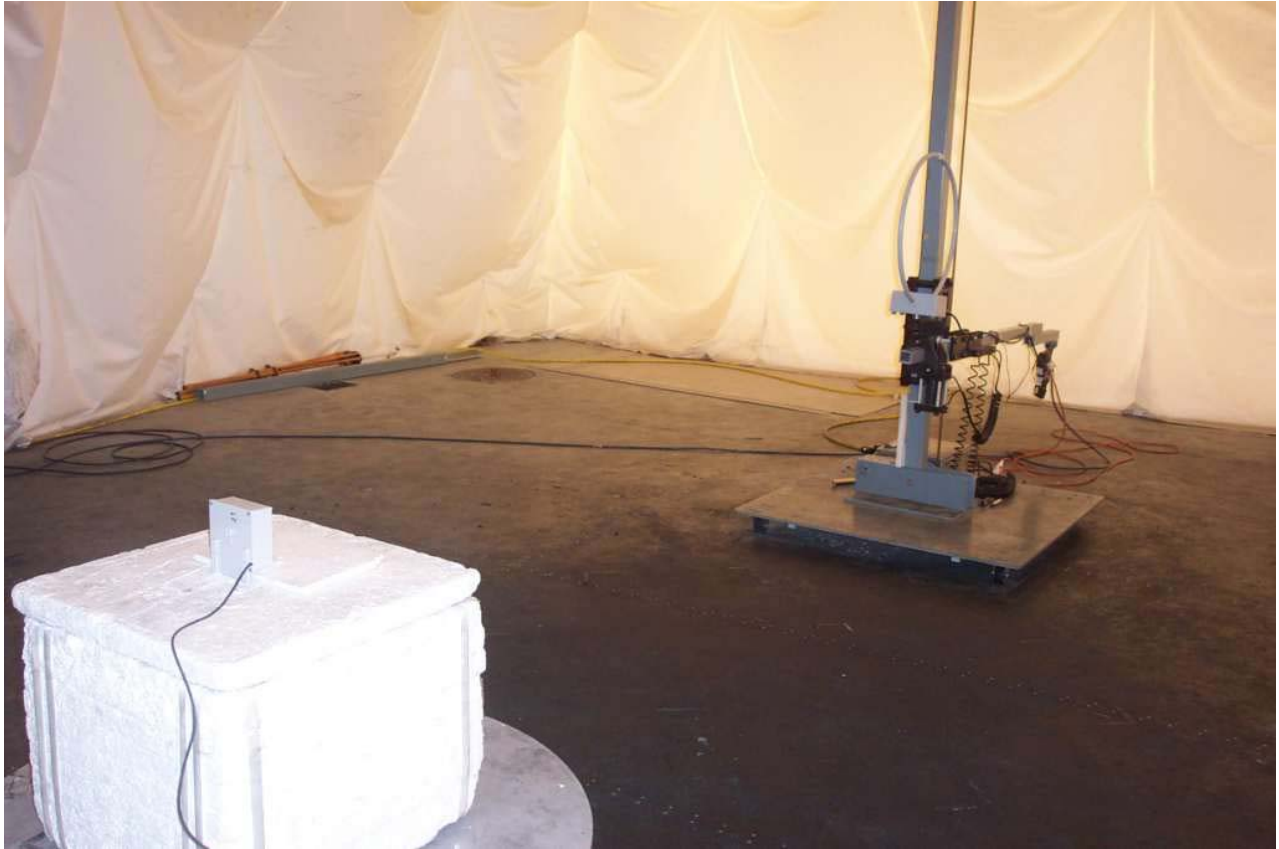
Figure 3: Test setup for radiated spurious between 9kHz and 30MHz with Loop Antenna shown with Remote.
