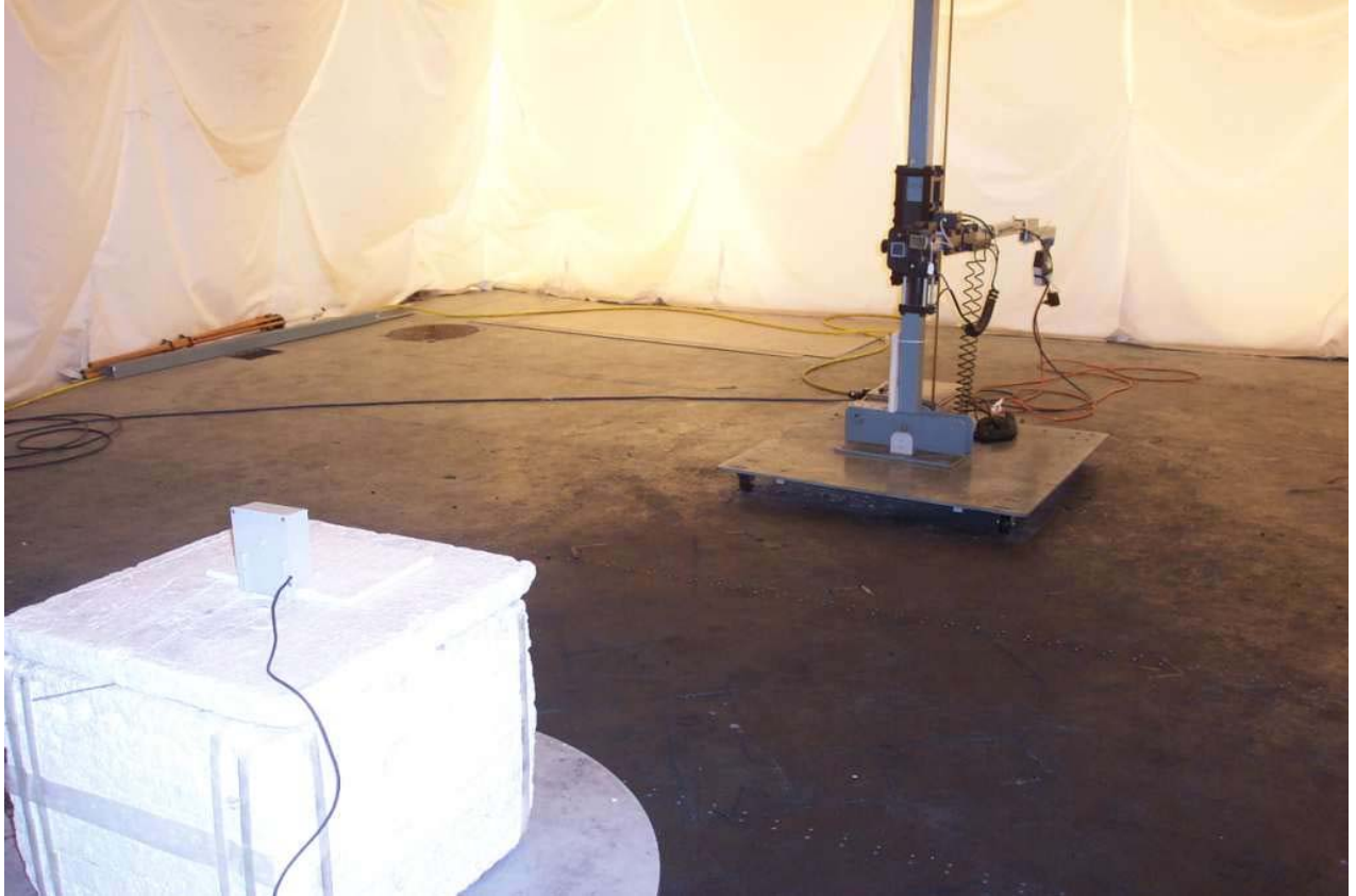
Figure 19: Test setup for radiated spurious emissions above 18GHz (Vertical polarity) shown with Remote on turntable
