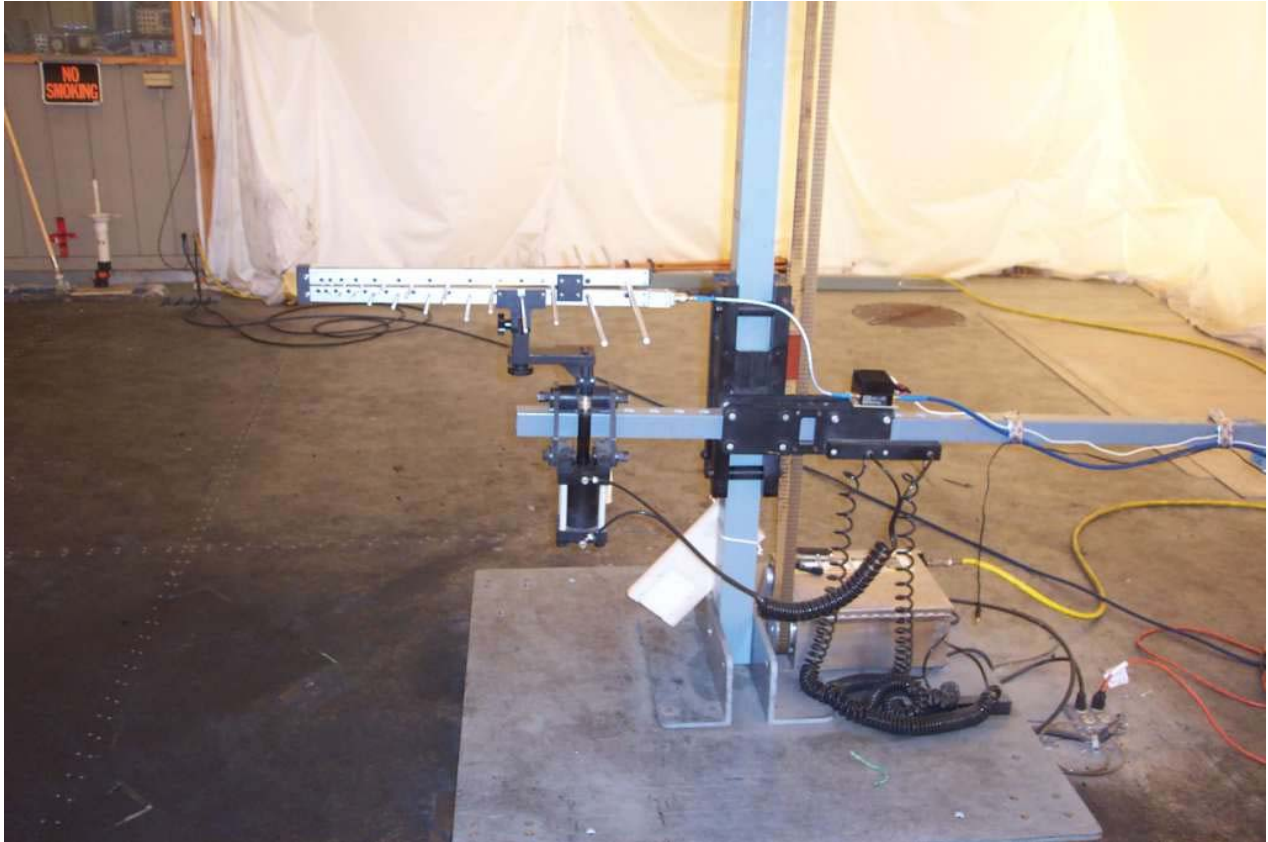
Figure 10: Test setup for TX radiated spurious between 200MHz and 2GHz with Log Periodic in horizontal orientation
