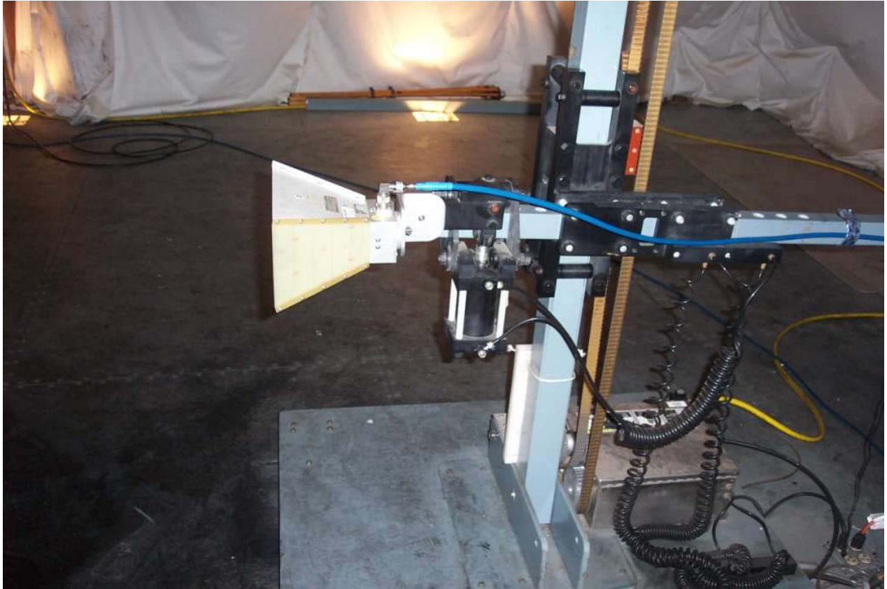
Figure 17: Test setup for TX fundamental radiated emission without high pass filter horn in vertical polarity
