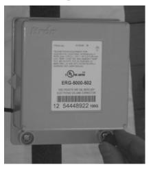
**3.** Push both tamper seals all the way into place with a 1/4-inch nut driver or similar tool.
