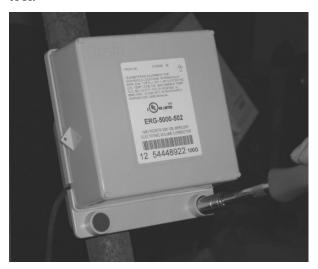
The 100G Remote ERT Module should look like this after the tamper seals have been installed.
