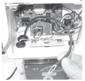
**3.** Install the Phoenix connector (supplied by Mercury). Connect the red, blue and white wires to the Phoenix connector terminals as directed in Code Settings on page 3.
