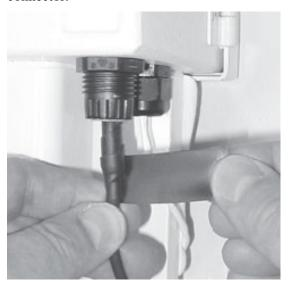
**6.** Install and tighten compression nut. This provides strain relief and seals the connection.
