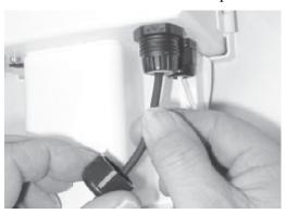
**2.** Strip one inch from the outer insulation and about 1/4-inch from the red, white and blue wires. Twist the blue and white wires together.
