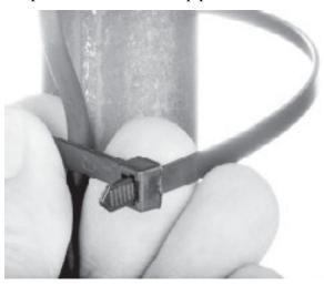
5. Pull the cable tie tight and cut off excess length. Dispose of the cut-off piece properly.
