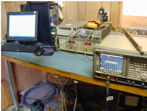
EMC analyzer with the Antenna correction Factor, Amplifier Gain, and Coax loss programmed into internal tables.
