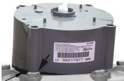
A gap may be caused by misalignment of the endpoint wiggler and meter wiggler's drive teeth. Pushing down on the endpoint could damage the endpoint wiggler or meter drive teeth. To eliminate a gap, remove the 100G Datalogging Gas Endpoint and repeat steps 2 and 3.
