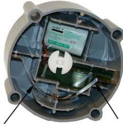
1. Tilt the 100G Datalogging Commercial Gas Endpoint at an angle and turn the wiggler until the drive notches line up with the meter wiggler's drive teeth.
