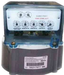
Index covers may (or may not) have tamper seal cups (on the back of the cover) for added security. Index removal assumes the installer will remove any tamper seals or wires before continuing with these instructions.
