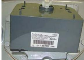
A gap may be caused by misalignment of the endpoint wiggler and meter wiggler's drive teeth. Pushing down on the endpoint could damage the endpoint wiggler or meter drive teeth. To eliminate a gap, slowly turn the 100G Datalogging Commercial Gas Endpoint's upper wiggler back and forth until the endpoint aligns with the meter's drive teeth.
