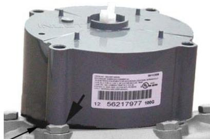
A gap may be caused by misalignment of the endpoint wiggler and meter wiggler's drive teeth. Pushing down on the endpoint could damage the endpoint wiggler or meter drive teeth. To eliminate a gap, slowly turn the endpoint's upper wiggler back and forth until the endpoint aligns with the meter's drive teeth.
