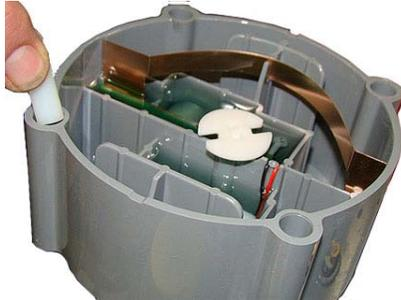
2. Turn the 100G Datalogging Commercial Gas Endpoint on its side and align the wiggler with the Itron-Actaris Commercial meter's drive dog.
