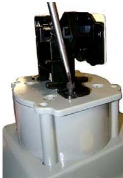
5. Place the index cover over the index with the clear side covering the index dials for easy reading. Align the holes in the index cover with the endpoint adapter plate mounting holes. Secure with the four mounting screws from the adapter kit. Tighten the mounting screws in a diagonal alternating pattern.
