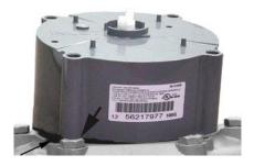
A gap may be caused by misalignment of the endpoint wriggler and meter wriggler's drive teeth. Pushing down on the endpoint could damage the endpoint wriggler or meter drive teeth. To eliminate a gap, remove the 100G Datalogging Gas Endpoint and repeat steps 2 and 3.
