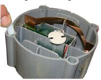
**2.** Turn the 100G Datalogging Commercial Gas Endpoint on its side and align the wriggler with the Itron-Actaris Commercial meter's drive dog.
