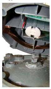
2. Align the endpoint so the screw holes line up with the meter's top screw holes. Carefully lower the endpoint on the meter with the wriggler notches lining up with the meter's wriggler teeth.
