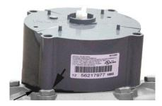
A gap may be caused by misalignment of the endpoint wriggler and meter wriggler's drive teeth. Pushing down on the endpoint could damage the endpoint wriggler or meter drive teeth. To eliminate a gap, slowly turn the endpoint's upper wriggler back and forth until the endpoint aligns with the meter's drive teeth.
