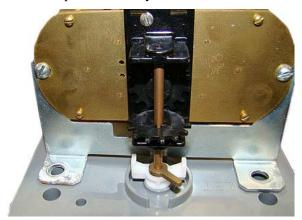
**5.** Install the index cover. For index covers with flat-surface screw holes, use screws (SCR-0062-002), flat washers (WSH-0020-005), and cork washers (WSH-0032-001). For index covers with tamper seal cups, use screws, (AS-568A-011, 5/16" ID x 7/16 OD) o-rings, and tamper seals.
