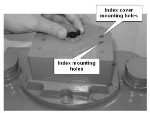
4. Rotate the 100G ERT Module drive to make sure it engages with the meter drive.
