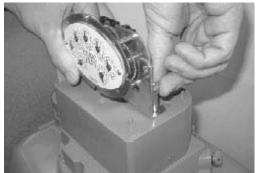
6. Turn each screw 1/4 to 1/2 turn after it contacts the mounting plate. If you are using a torque wrench, tighten to 72 inch-pounds.
