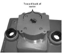
7. Place the extension driver onto the 100G ERT Module wriggler.
