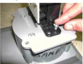
**8.** Gently place the index assembly onto the adapter plate and install the two index mounting screws.
