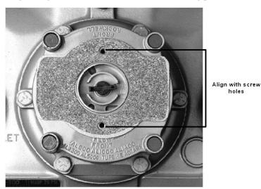
**3.** Turn the index wriggler so it will go across the ERT module wriggler when you put the index onto the mounting plate.
