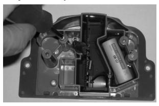
**3.** Place the index's mounting leg screw slot under the screw head and tighten the screw enough to hold the index leg in place, but loose enough so you can pivot the index around the screws.
