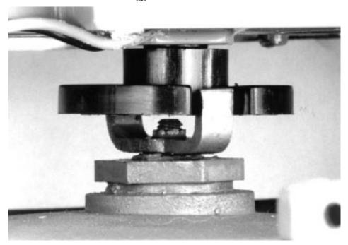
**4.** Make sure there is no gap between the bottom of the ERT module and the top of the meter. If there is a gap, it is because the drive notches of the ERT module's lower wriggler are not properly aligned with the meter wriggler's drive teeth.
