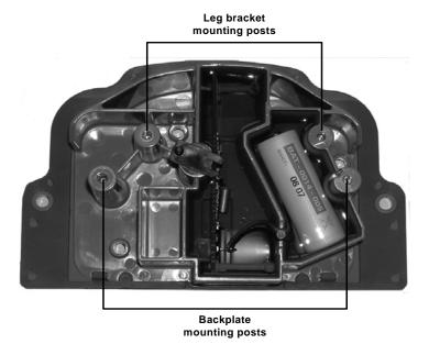
Indexes that have mounting legs as well as holes for mounting without legs can be mounted by using SCR-0015-001 to attach the mounting legs or by removing the two mounting legs and using SCR-0037-001 to attach the index to the ERT modules' index backplate mounting posts.
