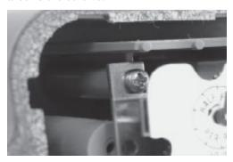
**4.** Make sure the index's right mounting leg screw slot is positioned over the ERT module's right index mounting leg screw hole.
