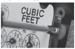
3. Turn each screw 1/4 to 1/2 turn after it contacts the index backplate.
