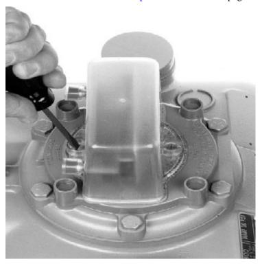
**3.** Remove the gasket from the index cover mounting plate and set it aside where it will not get damaged. You will use the gasket later in the installation.
