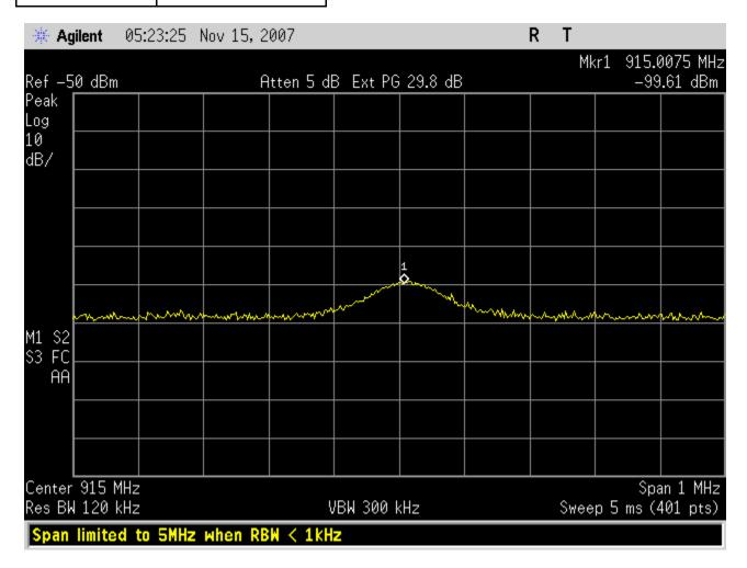
Receiver signal measured conducted with an amplifier gain of 29.8db.
