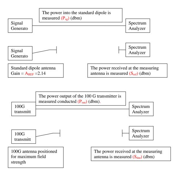
$A_{REF}$  = Antenna Gain of the standard dipole (dbi) A<sub>DUT</sub>=Antenna Gain of the 100G device (dbi)
