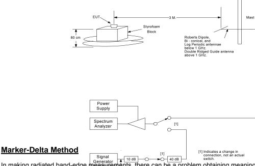
In making radiated band-edge measurements, there can be a problem obtaining meaningful data since a measurement instrument that is tunged to a band-edge frequency may also capture some in-band signals when using the resolution bandwidth (RB₩) required by measurement procedure ANSI C63.4-1992 (hereafter C63.4). In an effort to compensate for this problem, we have developed the following technique for determining band-edge compliance.
