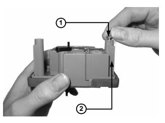
7. Place the index mounting screw slot under the screw head. *Do not* tighten the screw yet.
