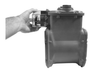
**4.** Install and tighten all ERT module assembly mounting screws, working in a diagonal pattern as shown below. Tighten the mounting screws to 15 to 20 inch-pounds of torque. Use the 1/4 - 20 x 5/8-inch screws for this step (you can use the original mounting screws if they were the correct size and not corroded; otherwise, use the correct size Replacement Screws on page 6).
