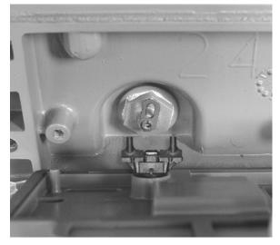
**3.** Gently place the ERT module assembly on the meter. Align the four screw holes on the ERT module assembly with the holes on the meter.
