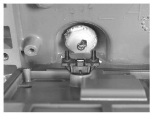
• For Two-Foot Meters: Align the ERT module assembly wriggler with the meter drive slot (as shown below). It is acceptable for the pin on the 100G wriggler to be installed inside or outside of the meter drive slot. For ease of assembly, Itron recommends that the pin on the 100G wriggler be installed outside of the meter drive slot.
