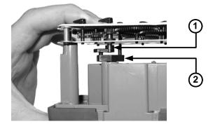
**9.** Install and tighten the left-hand index mounting screw (for indexes with either mounting screw slots or holes). Use one 8 - 32 x 3/16-inch screw for this step (you can use an original mounting screw if it was the correct size and not corroded; otherwise, use the correct size replacement screw).
