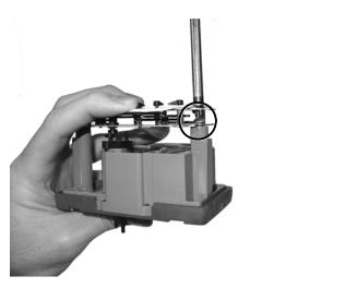
6. If the index has mounting screw *slots*, screw an index mounting screw (1) one to two turns into the ERT backplate's right-hand index mounting post (2). Use one 8 - 32 x 3/16-inch screw for this step (you can use an original mounting screw if it was the correct size and not corroded; otherwise, use the correct size replacement screw).
