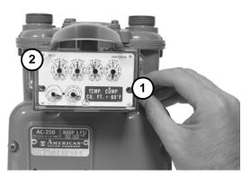
**6.** Press the new tamper seals into place using the 11/32-inch nut driver (or another similar blunt tool).
