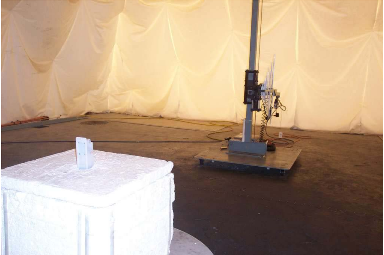
Photo 9: Test setup for radiated spurious between 200MHz and 2GHz with EMCO 3148 Log Periodic in vertical orientation shown with Range Extender in foreground
