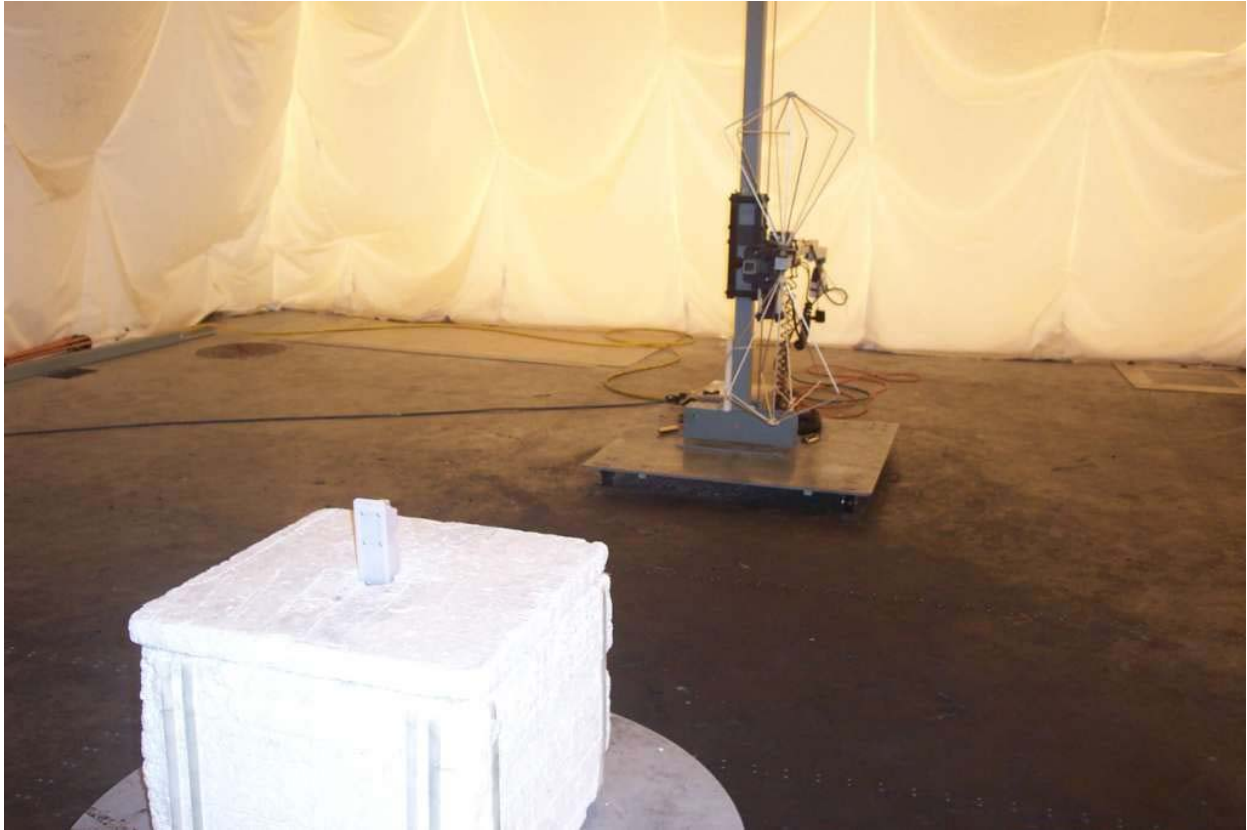
Photo 5: Test Setup for Radiated Spurious measurements between 30MHz and 300MHz using EMCO 3110B Biconical antenna shown here in vertical orientation and Range Extender in foreground
