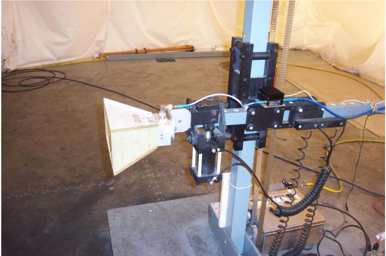
Photo 12: Test setup for TX radiated spurious emissions between 1 and 3GHz with MiniCircuits ZHL 1042J amp and EMCO 3115 horn antenna in vertical polarity (no highpass filter)
