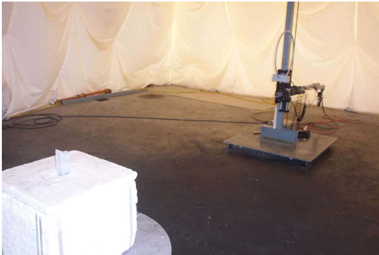
Photo 1: Test setup for radiated spurious between 9kHz and 30MHz with EMCO 6502 Loop Antenna shown with Range Extender
