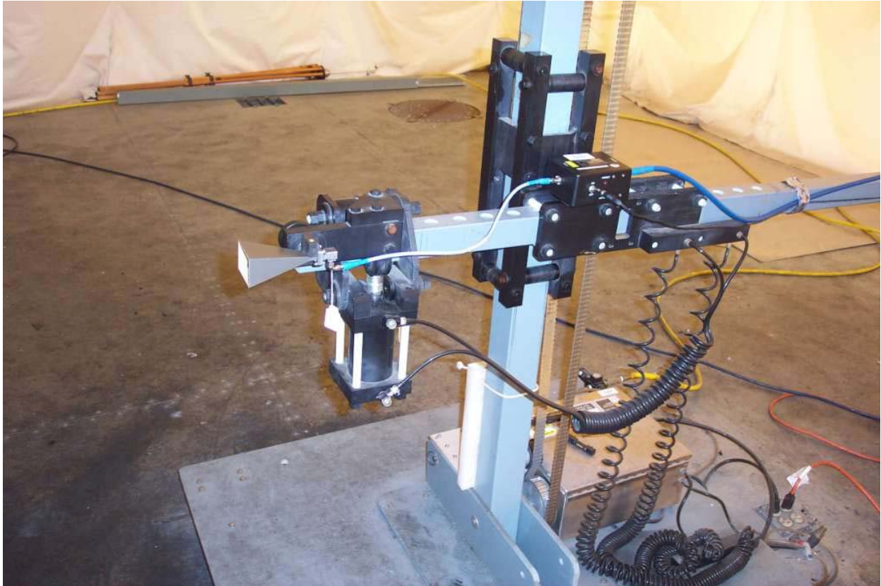
Photo 18: Test setup for radiated spurious emissions above 18GHz with PAM 0126 amplifier and AH systems SAS-572 Horn antenna in vertical polarity (high pass filtering is accomplished with horn antenna)
