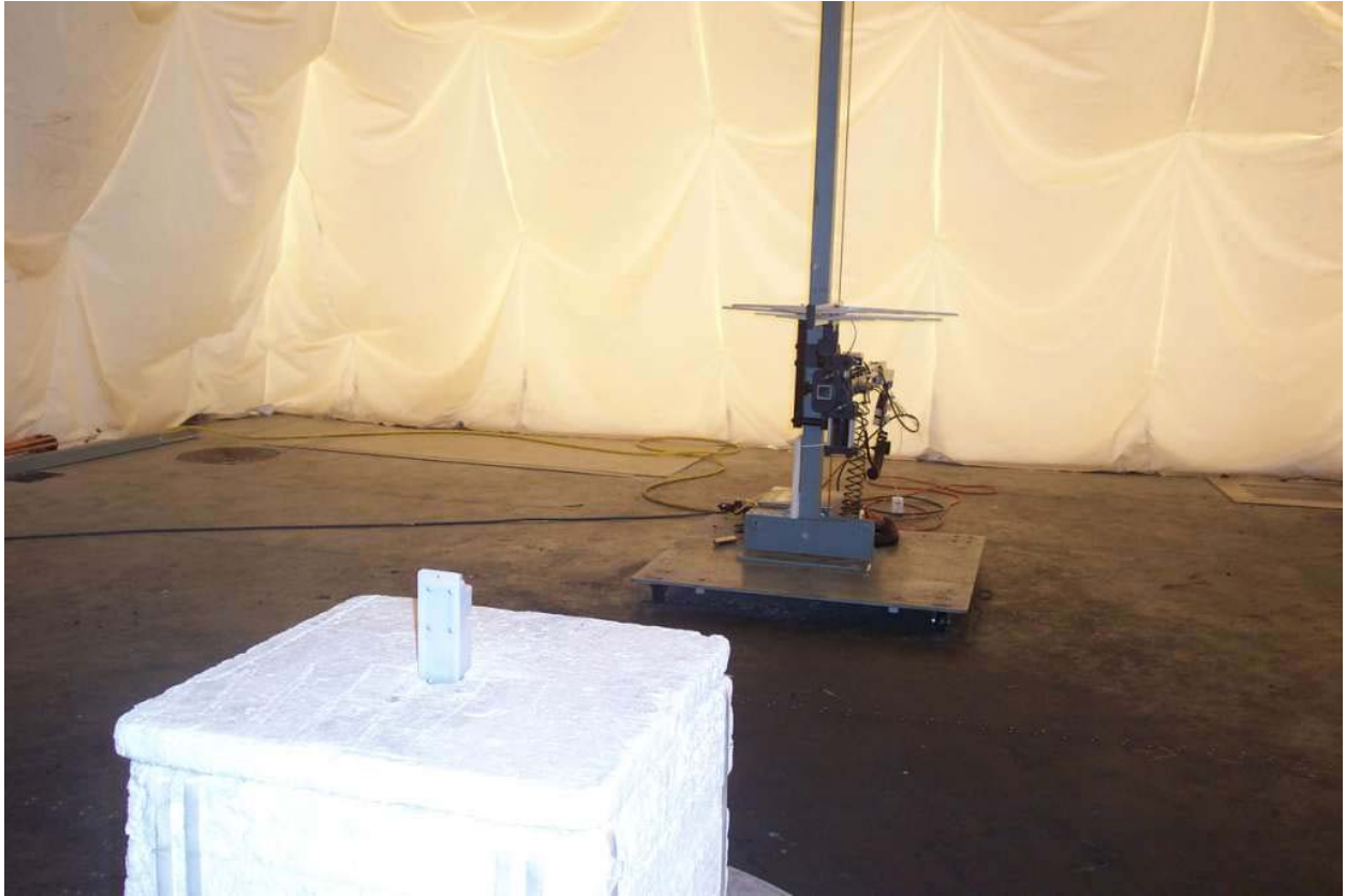
Photo 10: Test setup for radiated spurious between 200MHz and 2GHz with EMCO 3148 Log Periodic in horizontal orientation shown with Range Extender in foreground
