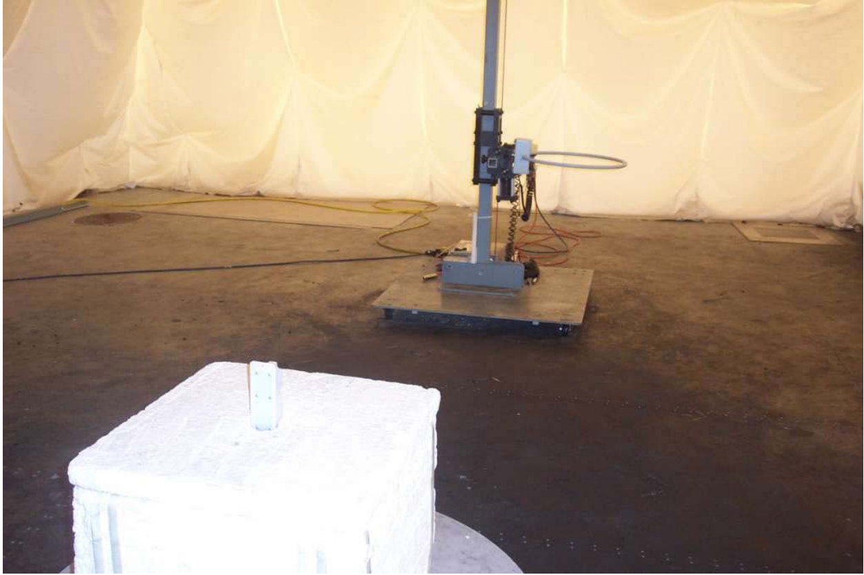
Photo 3: Test setup for radiated spurious between 9kHz and 30MHz with EMCO 6502 Loop Antenna shown with Range Extender
