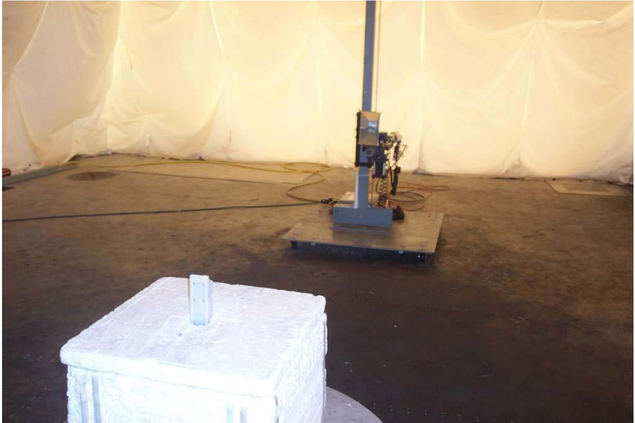
Photo 15: Test setup for radiated spurious emissions between 1 and 18GHz with EMCO 3115 horn antenna in horizontal polarity and Range Extender on turntable
