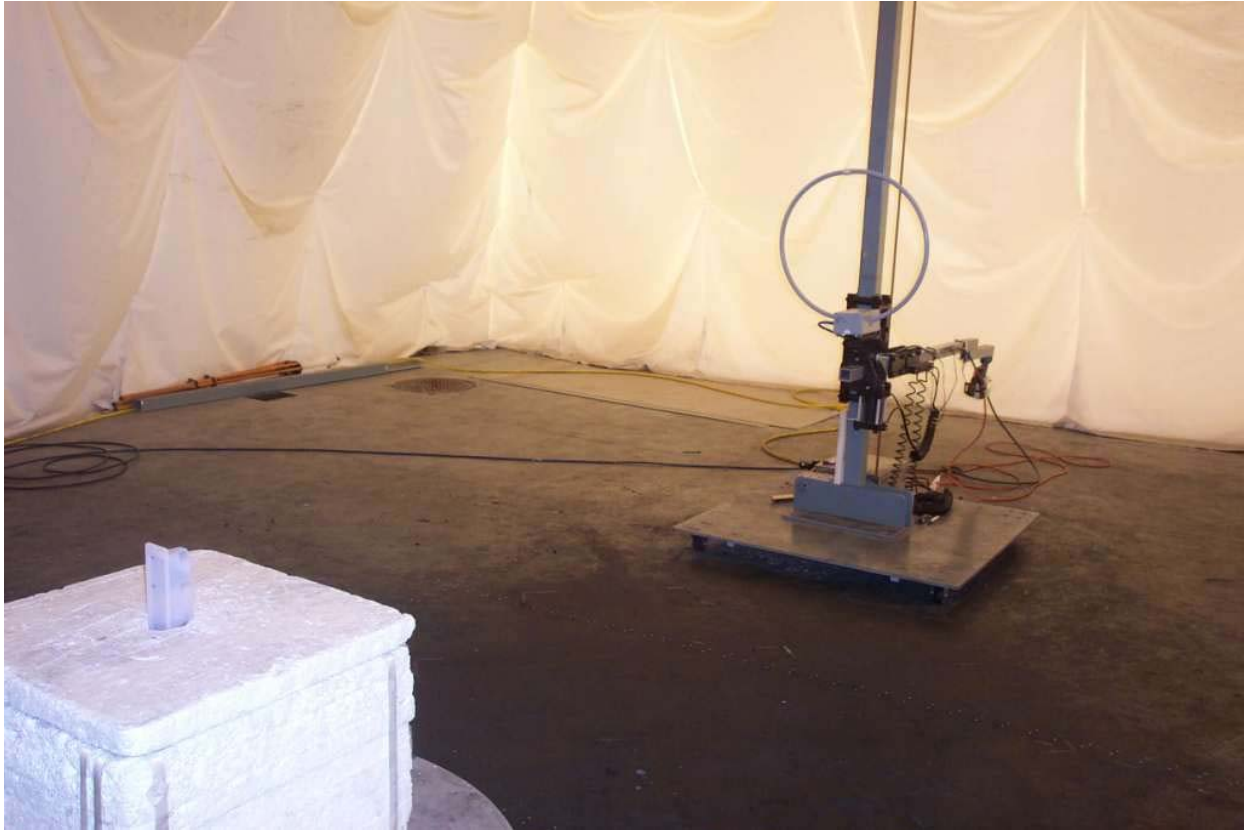
Photo 2: Test setup for radiated spurious between 9kHz and 30MHz with EMCO 6502 Loop Antenna shown with Range Extender
