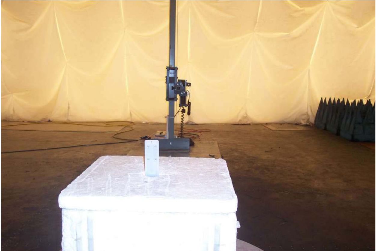
Photo 19: Test setup for radiated spurious emissions above 18GHz with AH Systems SAS-572 horn antenna in vertical polarity and Range Extender on turntable
