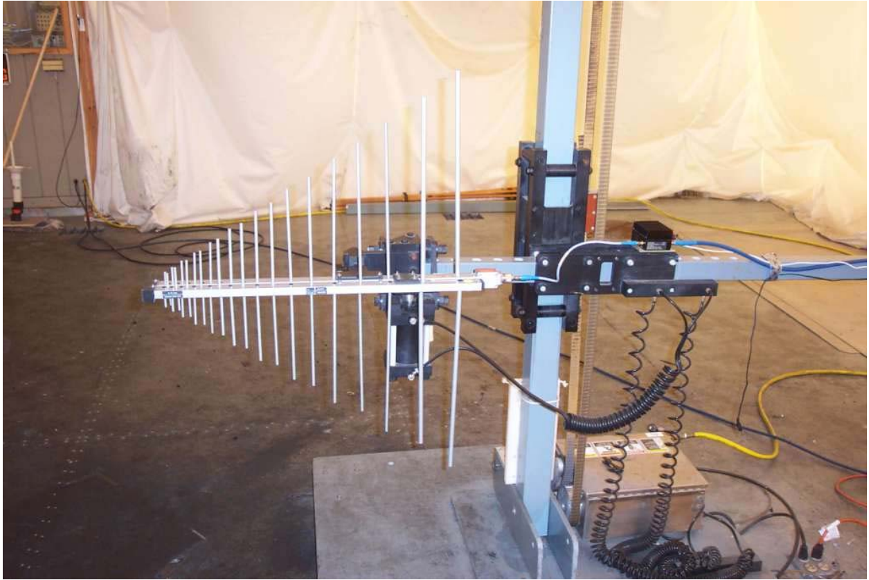
Photo 8: Test setup for TX radiated spurious between 200MHz and 2GHz with MiniCircuits ZHL 1042J amplifier and EMCO 3148 Log Periodic in vertical orientation
