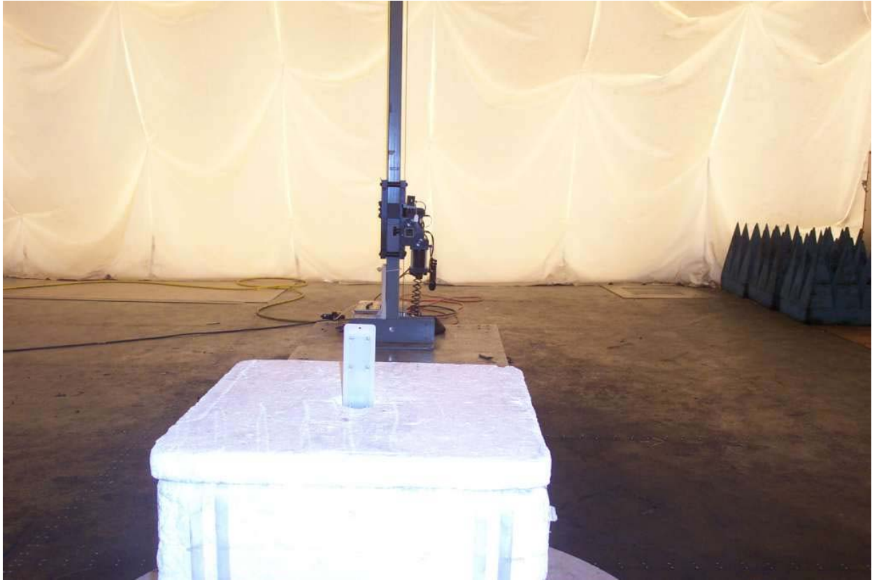
Photo 20: Test setup for radiated spurious emissions above 18GHz with AH Systems SAS-572 horn antenna in horizontal polarity and Range Extender on turntable
