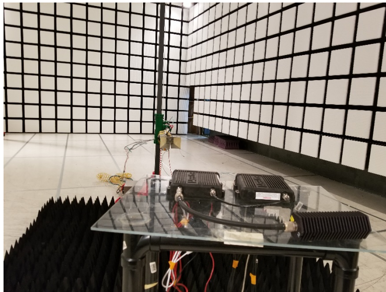
Figure 1.1-4: Radiated Emissions 1-2GHZ setup photo
