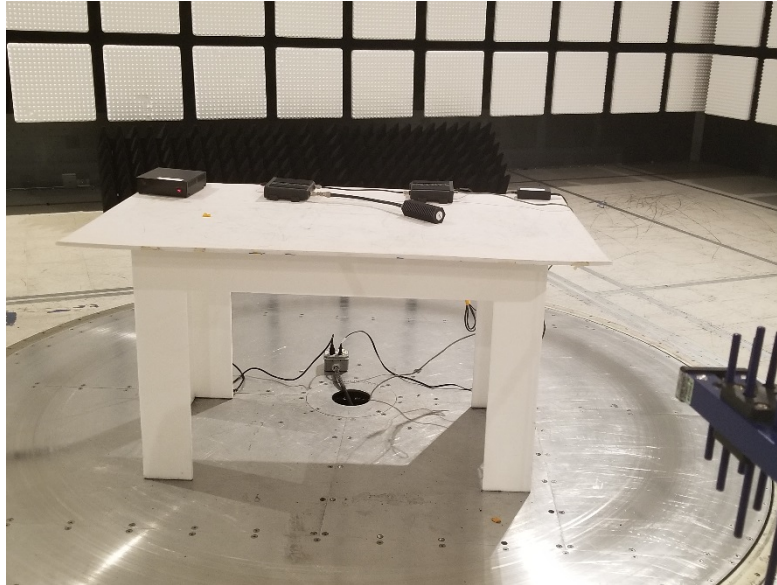
Figure 1.1-3: Radiated Emissions 30MHz-1GHz setup photo
