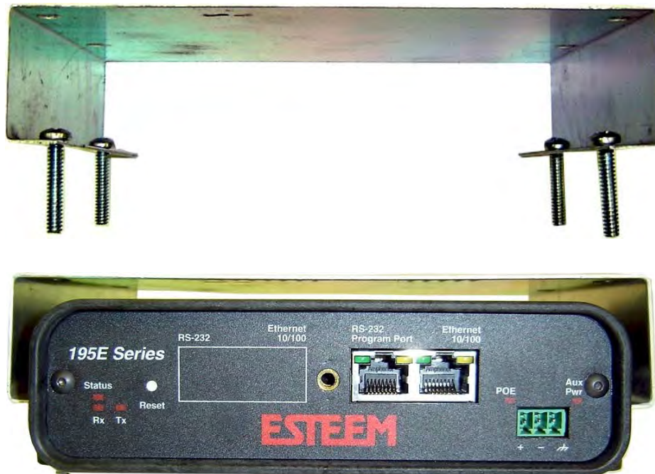
Figure 7: Heat Shield Attachment
