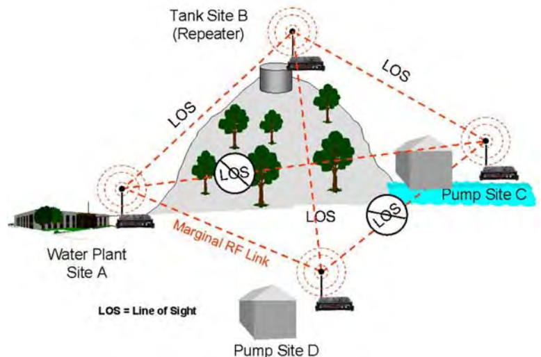
Figure 2: Small Mesh Network Diagram
