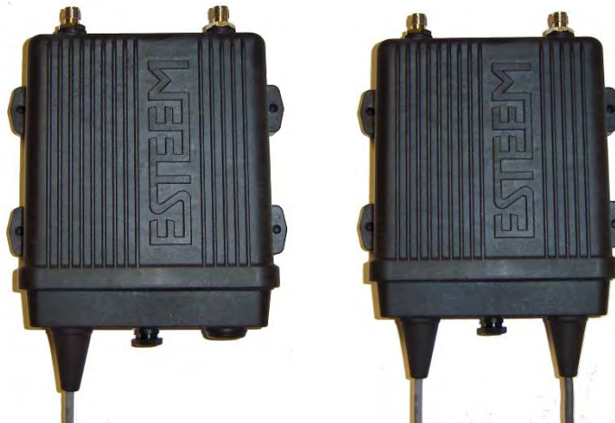
Figure 12: Face Plate Cover Installed on ESTEem
