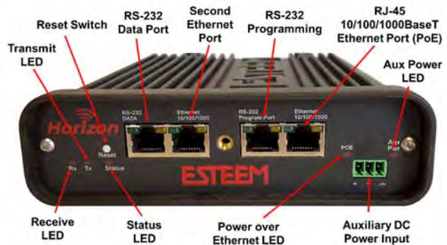
Figure 4: Horizon Front Panel Overview
