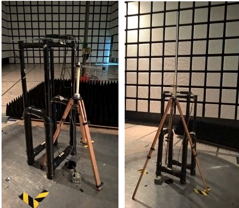
Figure 3.6-2: Radiated Emissions Test Setup – above 1GHz
