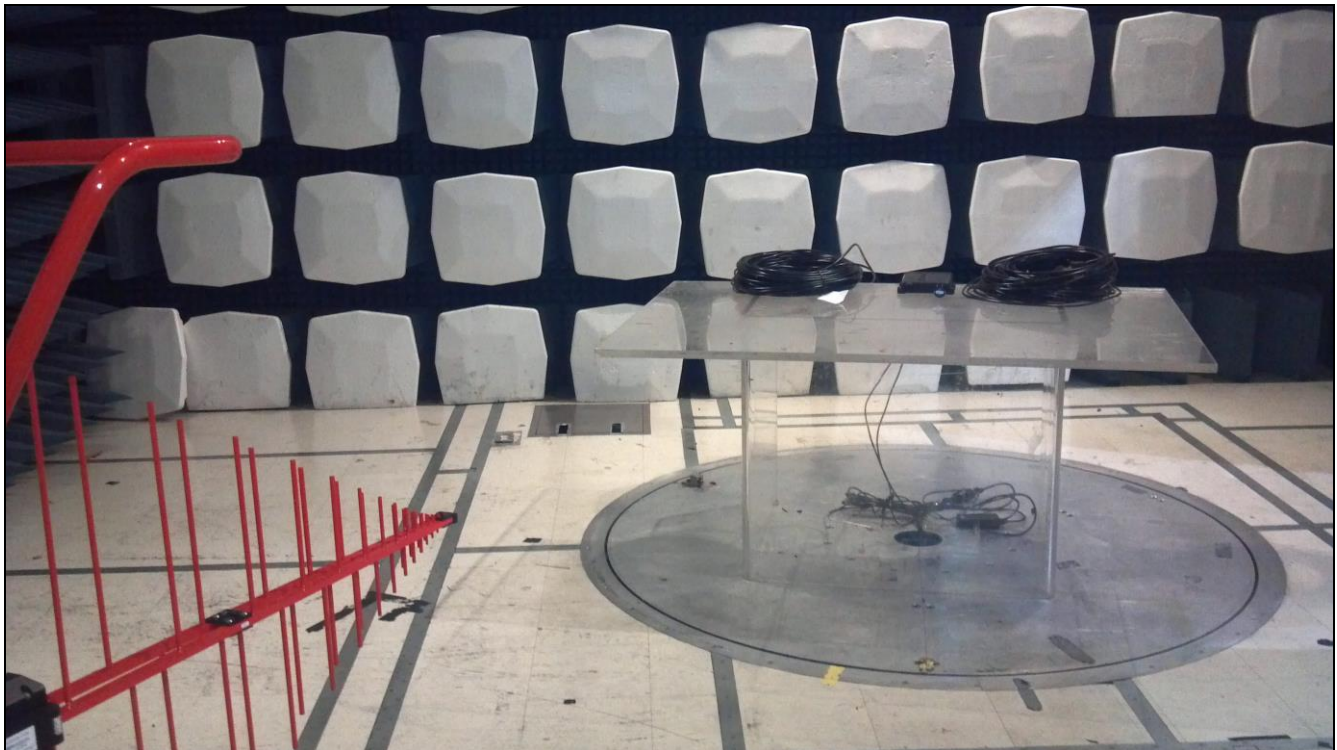
Photograph 2. Radiated Emissions, 30 MHz – 6 GHz
