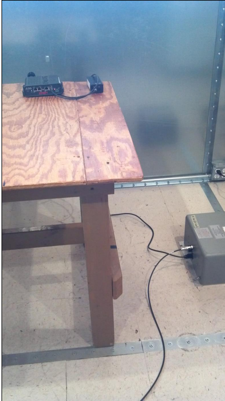
Photograph 1. Conducted Emissions, Test Setup
