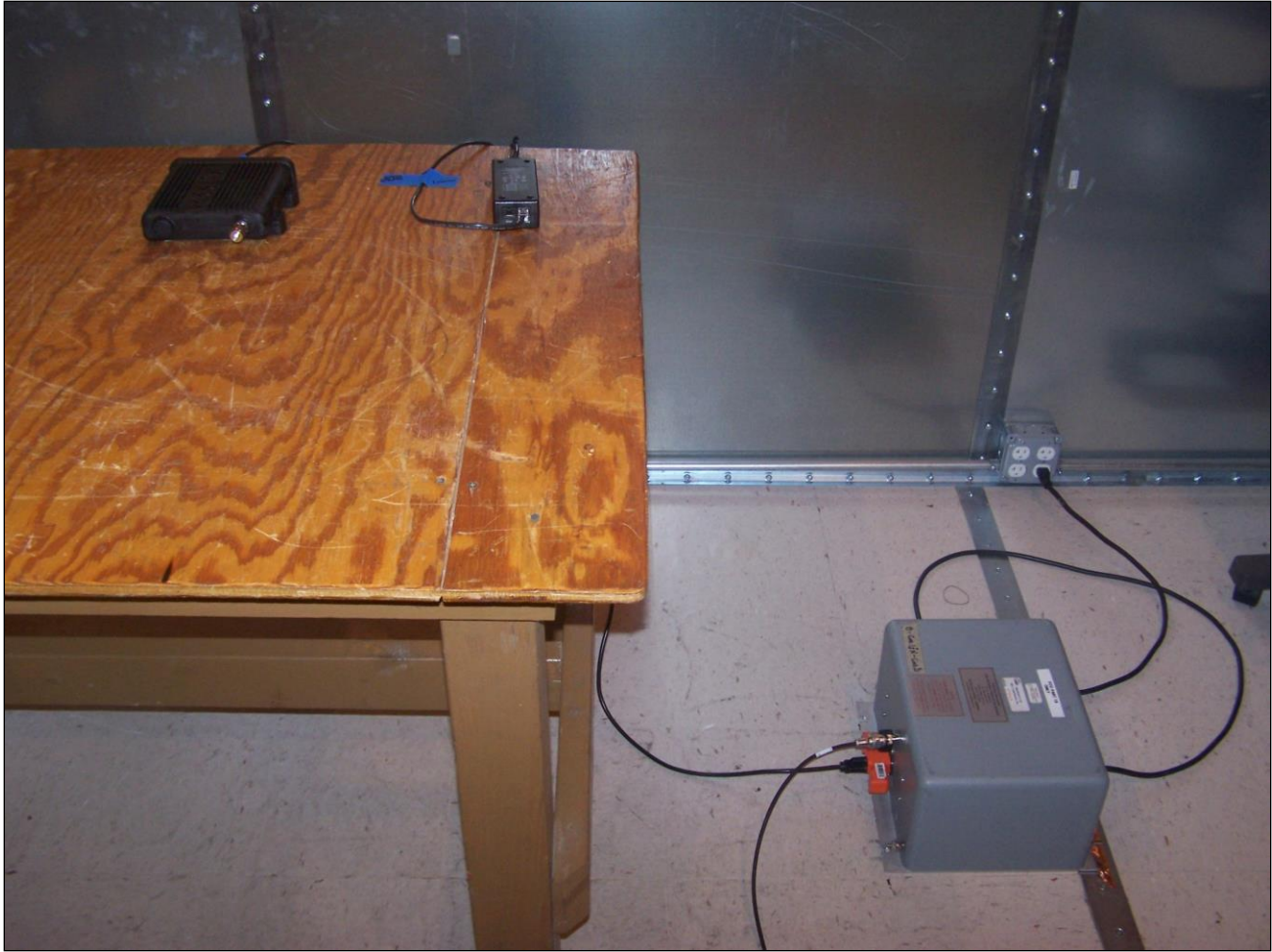
Photograph 1. Conducted Emissions, Test Setup
